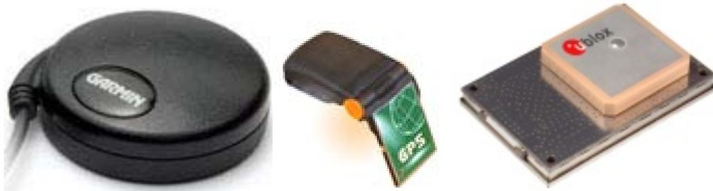
**Figure 3: Example Commercial GPS Receivers**
