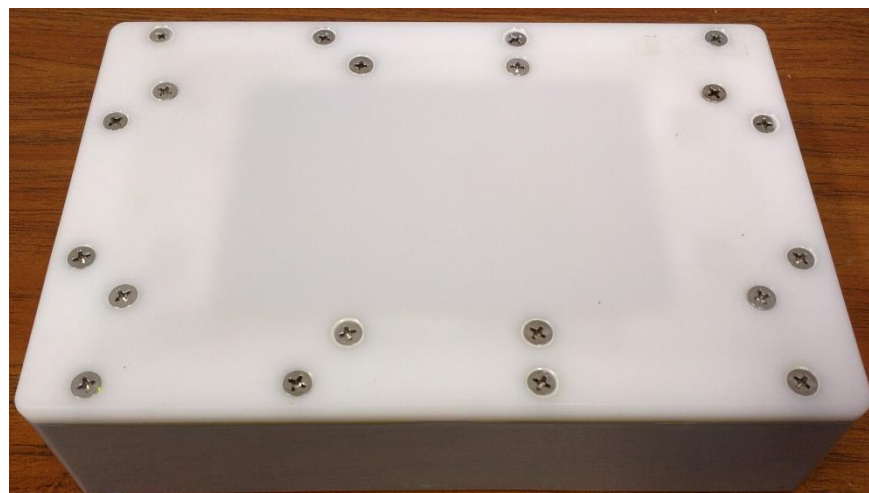
Figure 3.2: Heated enclosure ver. 1.2. AHMCT added mechanical fasteners to prevent delamination in the event of adhesive failure between the aluminum enclosure and the Delrin fascia
