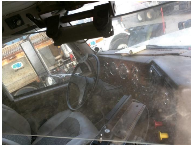
Figure 2.1: The 0024 snowplow combiner before cleaning
