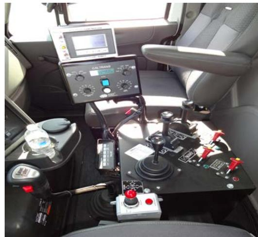
*Stock Caltrans Tow Plow In-Cab Testing Controls*
