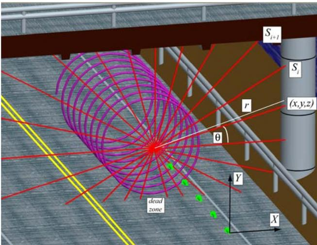
Figure 2 – Bridge profile scan geometry
