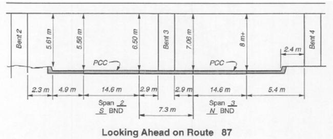
Figure 4 – Sample Caltrans clearance diagram. Software to generate diagrams from the extracted data is in development.
