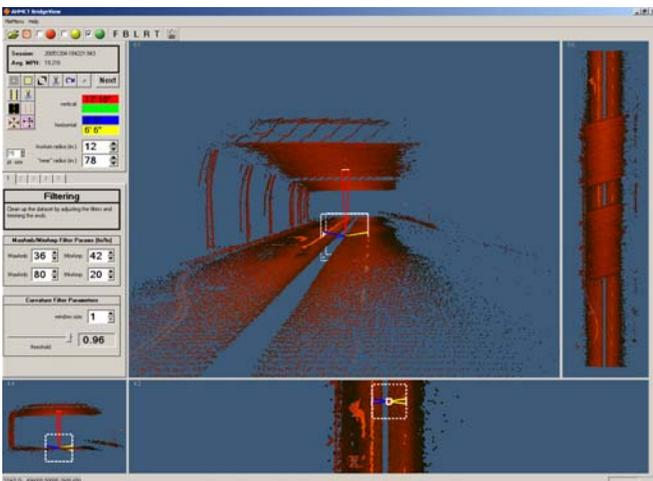
Figure 3 – Sample visualization software screen, showing tool for manual height and width dimension identification
