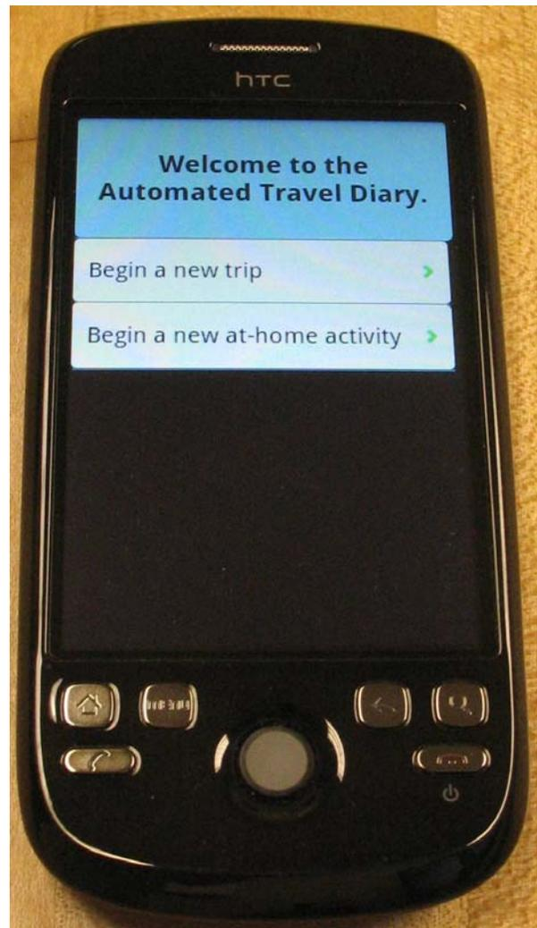
Figure 1 – The Phase 2 GPS-ATD on HTC Magic Phone
