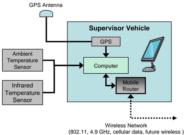
Figure 3 – Mobile information system in-vehicle configuration
