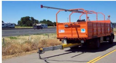
The Random Crack Sealer reduces worker exposure to traffic and transforms the strenuous task of pavement sealing into a simple computer point and click process.
