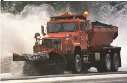
Three driver-guidance snowplows help Caltrans keep I-80 open despite extreme snow storms. Both GPS and roadway magnet guidance systems, along with radar systems and heads-up driver displays, have been developed by AHMCT.
