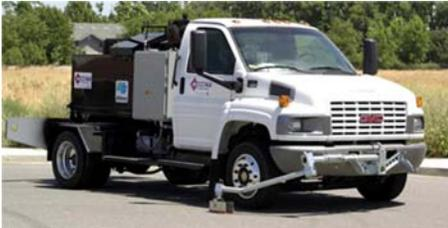
The logitudinal crack sealer is a truck with a trailer based sealant transfer nurse kettle. It was developed for longitudinal-only, high-production hot applied sealing at continuous speed with no direct worker exposure to traffic.
