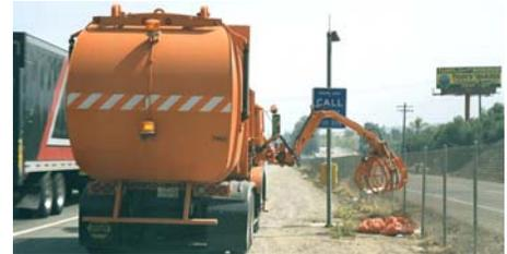
The Debris Removal Vehicle has a long, grasping arm which can pick up litter bags and large debris.
