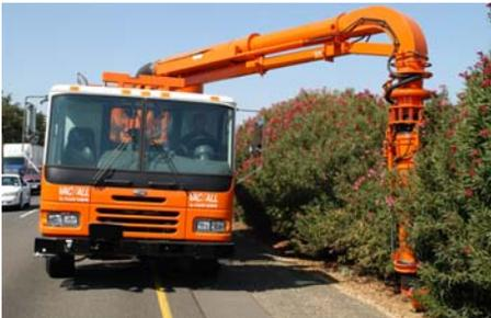
An articulated nozzle fits on existing vacuum vehicles to make it possible to suck debris from the roadside and behind guardrails.
