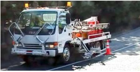
The Automated Cone Machine was developed and tested over several years, and the technology has led to a commercialized machine.
