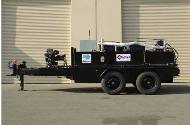
Figure 2 – TTLS Sealant Transfer Tank Trailer
