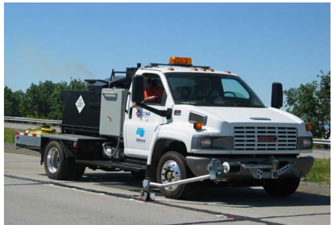
Figure 1 – TTLS Sealant Application Truck
