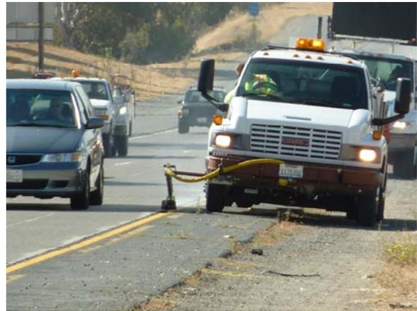
Figure 1 – Sealzall, Longitudinal Sealing Configuration
