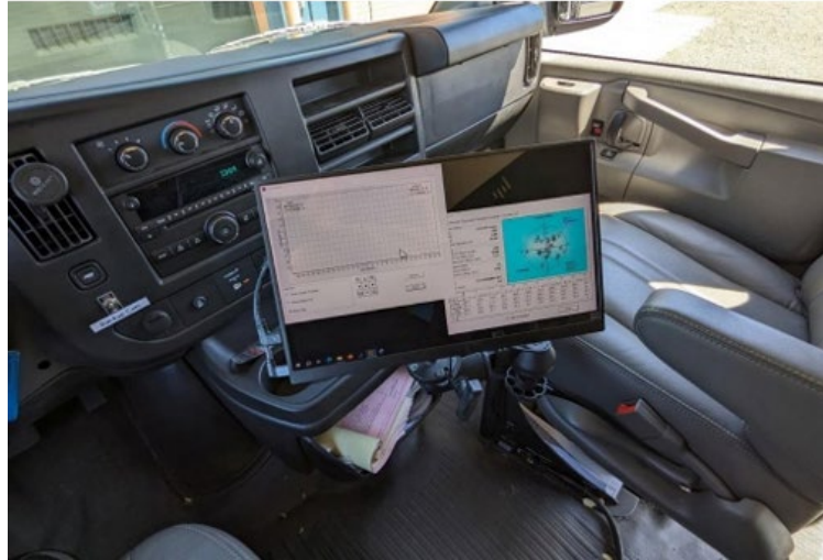
Upgraded front vehicle display showing the vehicle trajectory and GNSS satellite availability
