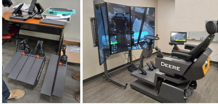
Figure 4.2: Left: exchangeable modules of John Deere simulator; right: installed John Deere simulator
