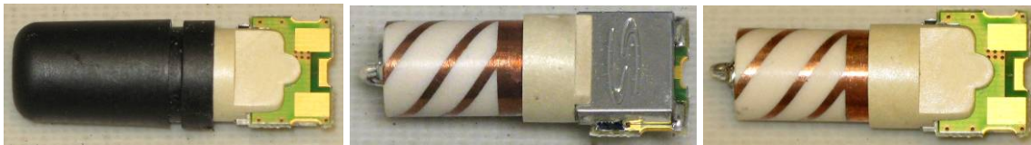
Figure 13: Sarantel GeoHelix GPS antenna
