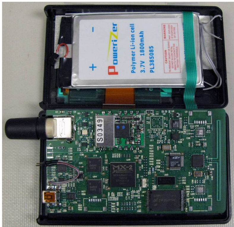
Figure 25: Fully-assembled GPS-ATD unit internals
