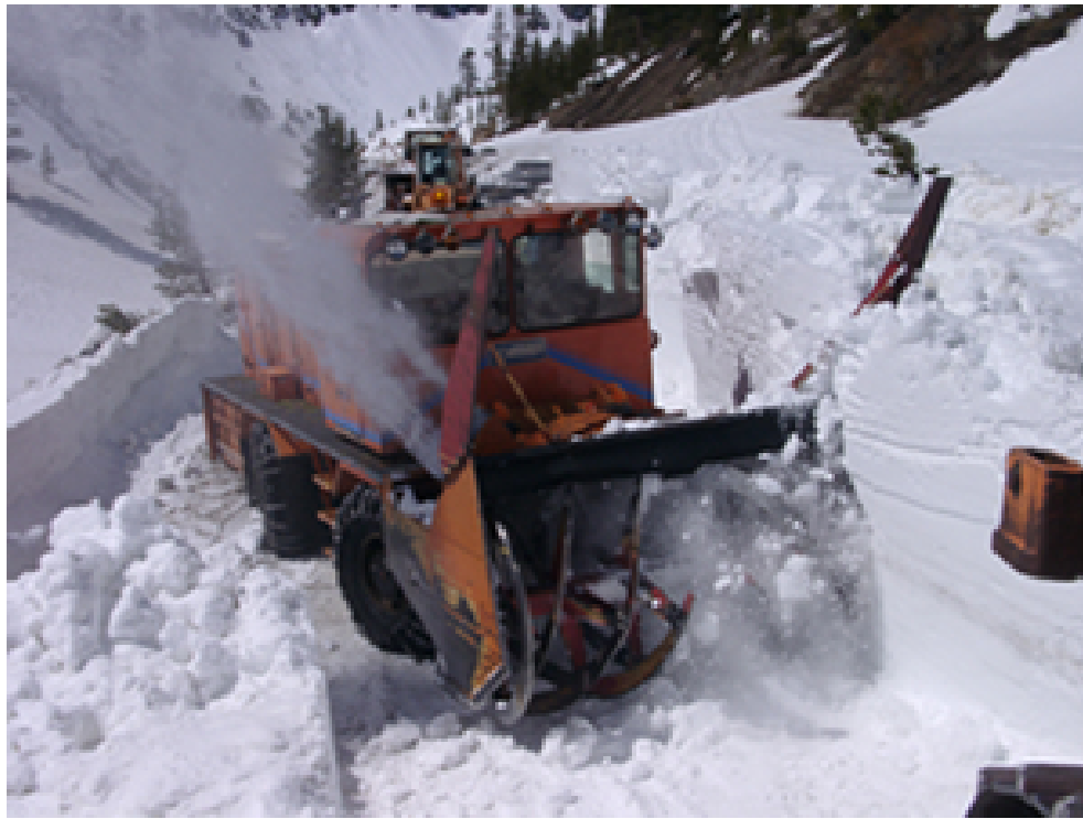
Figure 1.4: Rotary plow operating over the roadway during mountain pass opening
