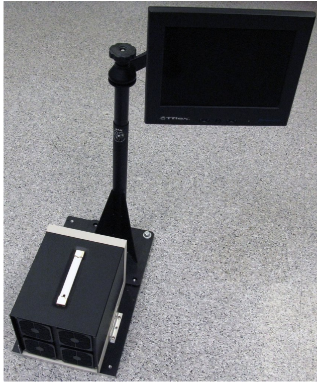
Figure 4.2: LCD, and System box containing computer and GPS receivers
