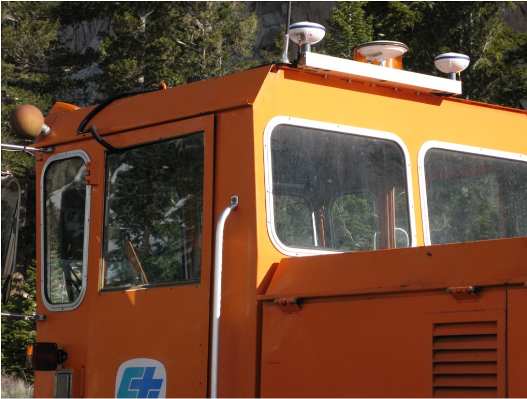
Figure A.1: Close-up view of antenna bar installation
