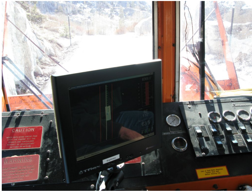
Figure 5.4: System installation showing LCD screen location
