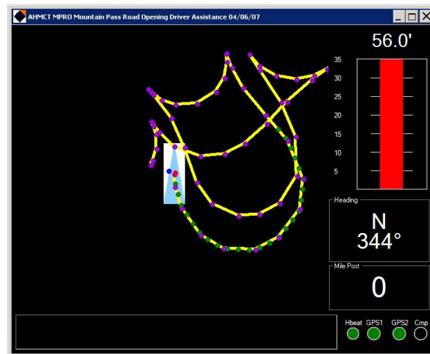
Figure 5.3: On-road testing of the heading subsystem, including backing maneuvers
