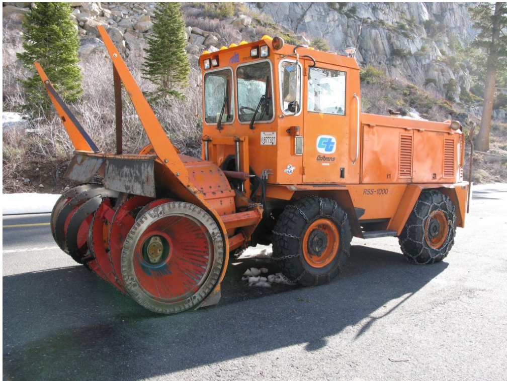
Figure 4.1: Caltrans rotary snow plow used for road opening operations
