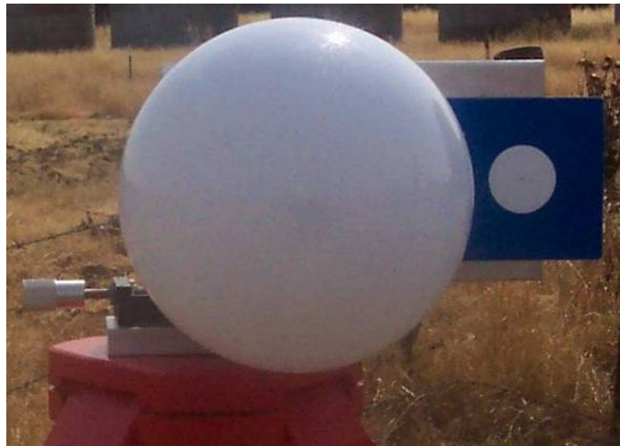
Figure 25: Angular Accuracy test fixture with Leica-specific target
