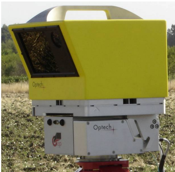
Figure 16: Optech ILRIS-3D System with motorized panning and tilting base
