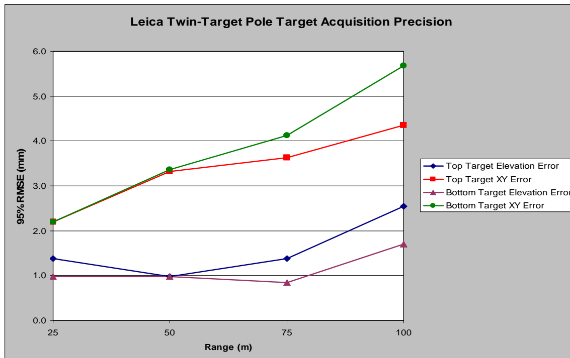
Figure 60: Leica Twin-Target pole target acquisition precision test results
