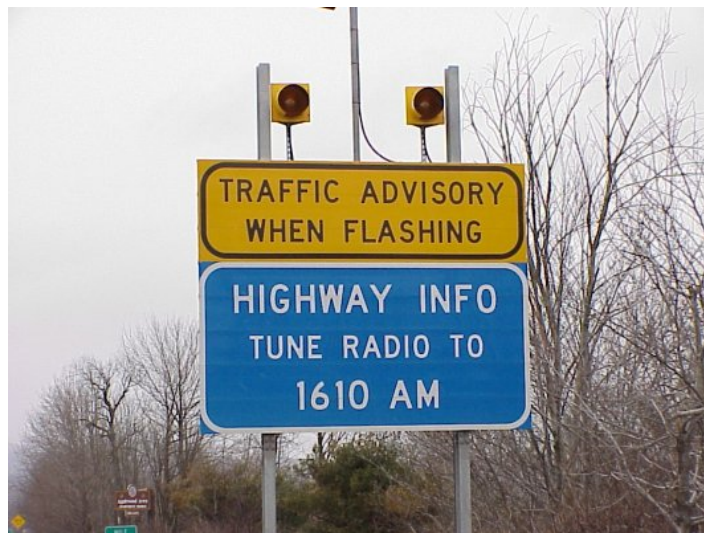
Figure 9.1: HAR sign and flashing beacons
