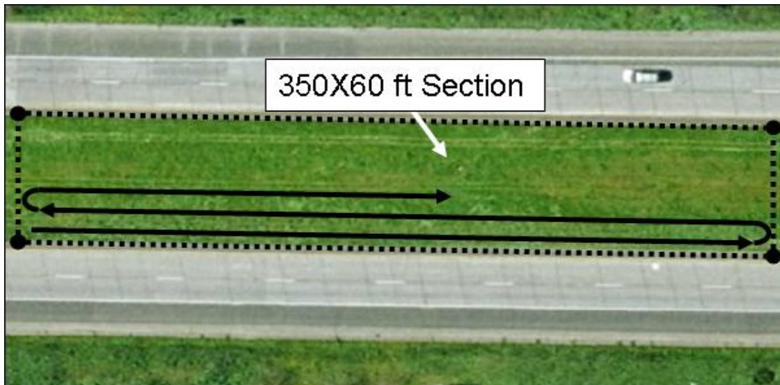
Figure 4.13 Anticipated mowing pattern overlaid on a section of HW-113 near Davis (Picture from Google Earth)
