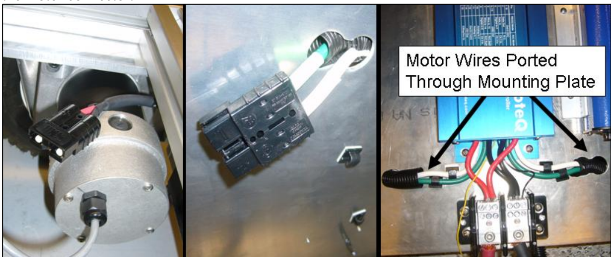
Figure A.9 Motor connector (left), controller connector (center), controller with ported wires (right)
