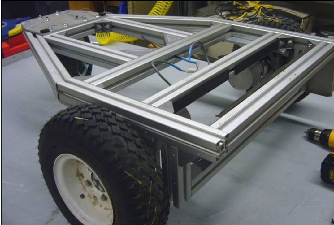
Figure 3.8 Testbed frame with mounted motors and wheels
