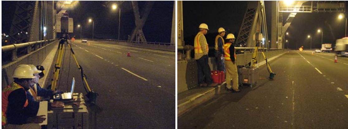
Figure 4: Night scanning of the old Bay Bridge for the design and construction of the new Bay Bridge detour
