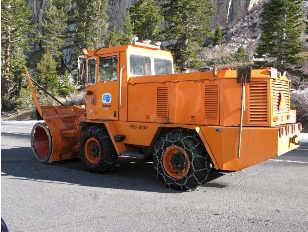
Figure 3.8: Caltrans rotary snow blower with GPS antenna bar
