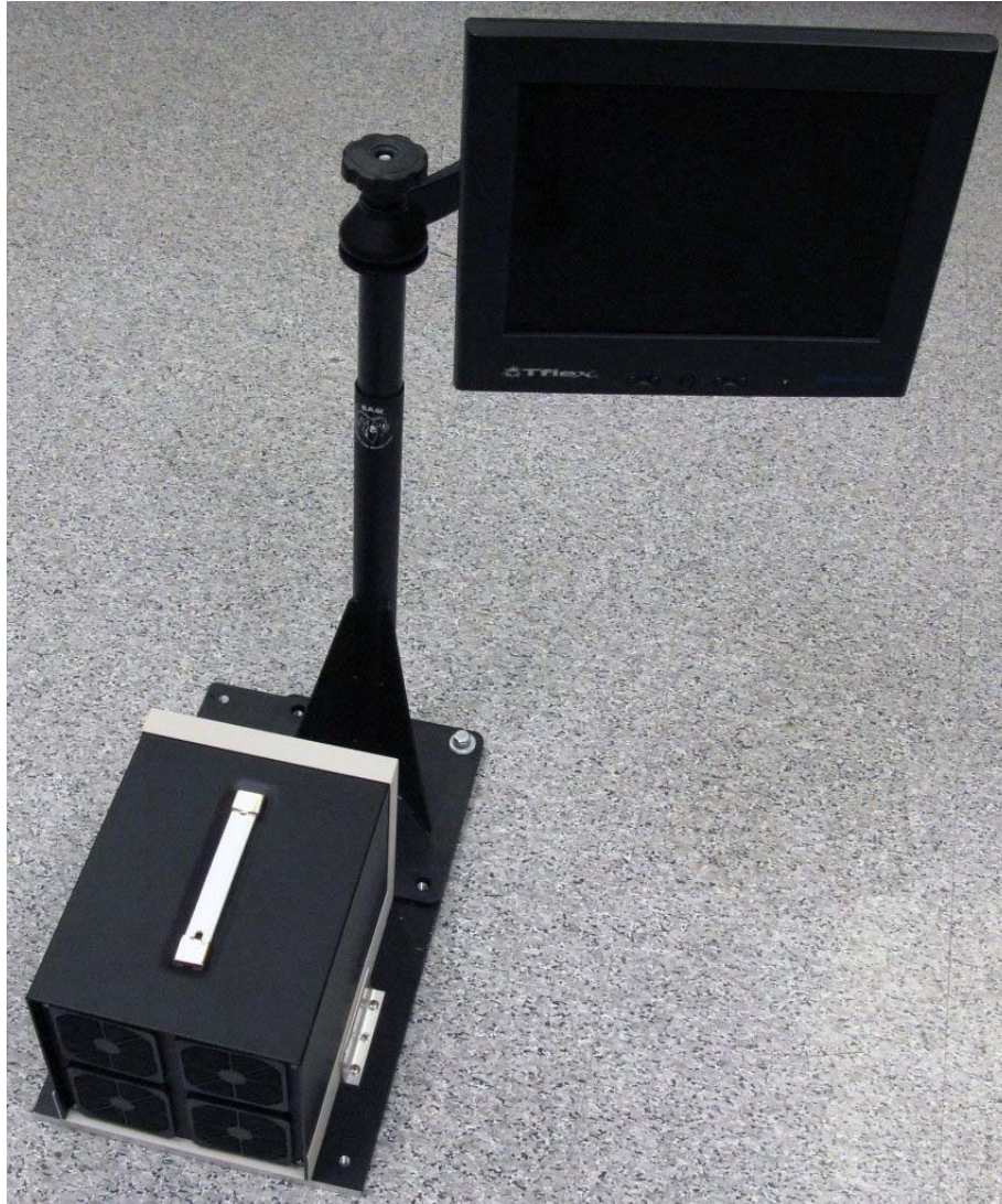
Figure 3.6: LCD, and system box containing computer and GPS receivers
