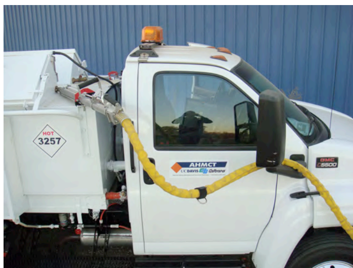
Figure 21. Sealant Hose Recirculation
