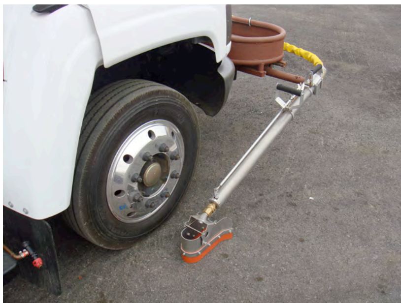
Figure 33. Longitudinal Sealing Shoe
