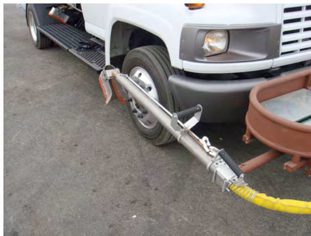
Figure 30. Wand Longitudinal Mounting
