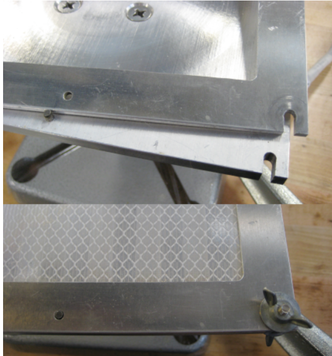
Figure 3-8: Detail of test bed showing frame attachment method
