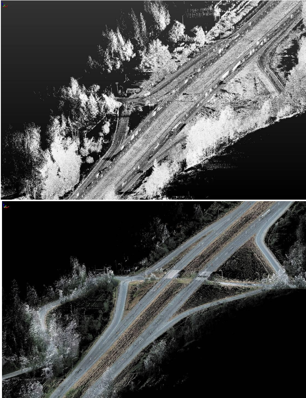
Figure 2.4: Point cloud of SR 167 pilot study site by two different systems (Courtesy of GeoMetrix Office)
