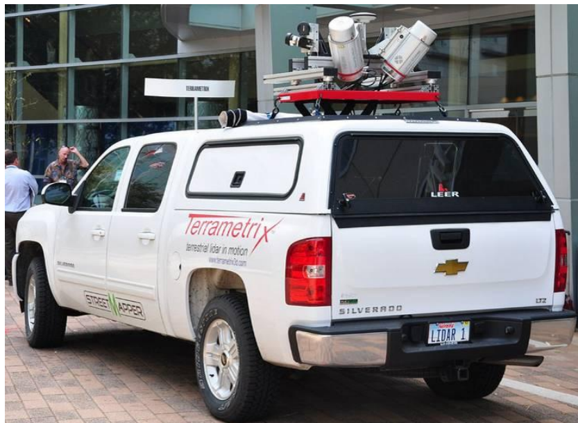
Figure A.19: StreetMapper 360 system mounted on a Terramatrix vehicle (copyright The American Surveyor Magazine© 2011)
