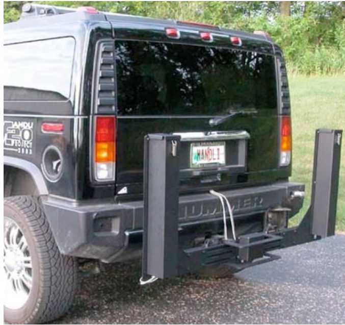
Figure 3.2 Hitch-mounted Vertical Clearance Measurement System (courtesy of Mandli Communications Inc.)
