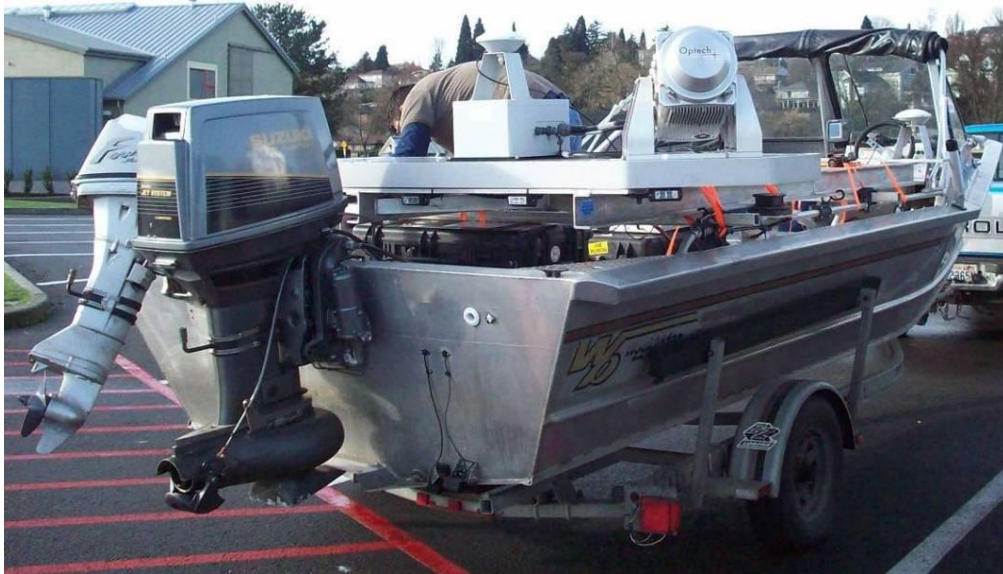
Figure A.15: Optech Lynx mobile LiDAR system mounted on a boat (Courtesy of GeoMetrix Office)
