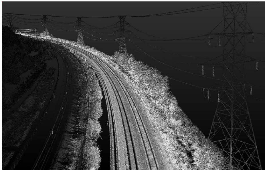
Figure A.18: Point-cloud produced by RIEGL VMX-250 system
