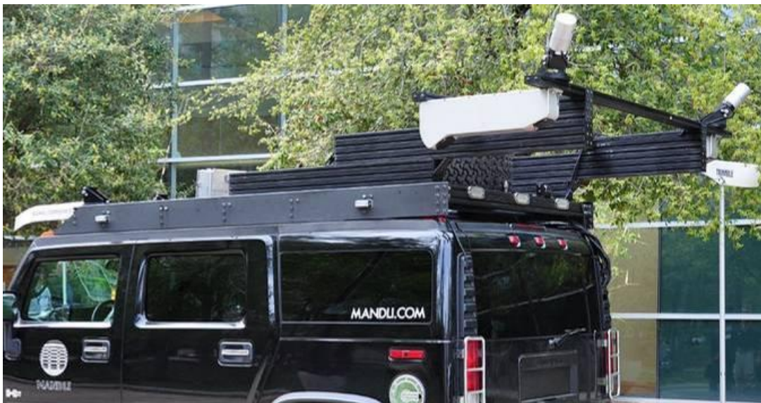
Figure A.12: Mandli Communications mobile LiDAR system with two Velodyne HDL-32E LiDAR scanners (copyright The American Surveyor Magazine© 2011)
