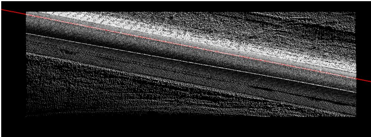
Figure 62: Automatic Line Extrapolation of Lane Line
