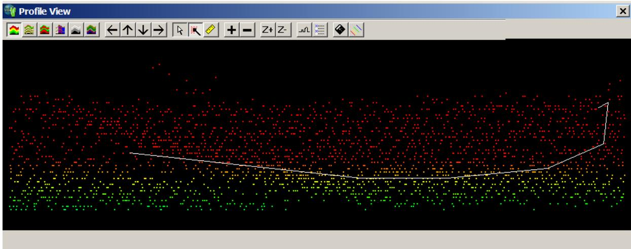
Figure 64: Manual Selection of points using Line Method in Profile View
