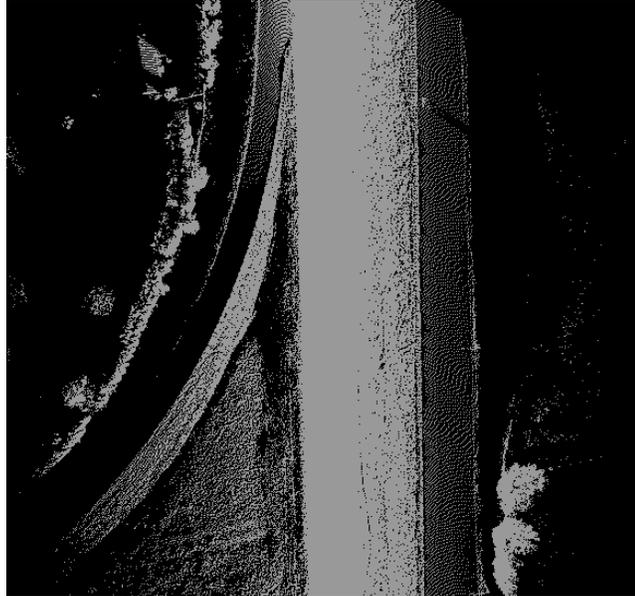
Figure 44: Point cloud classified to a ground class
