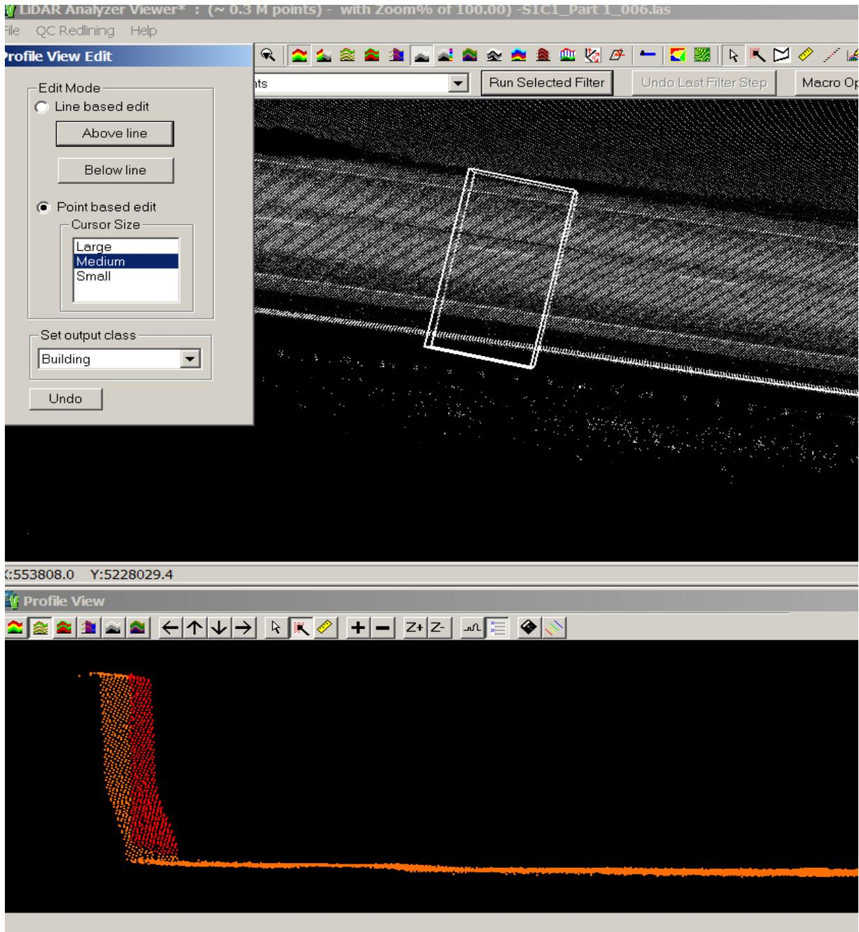
Figure 76: Selecting the points by moving the limit box
