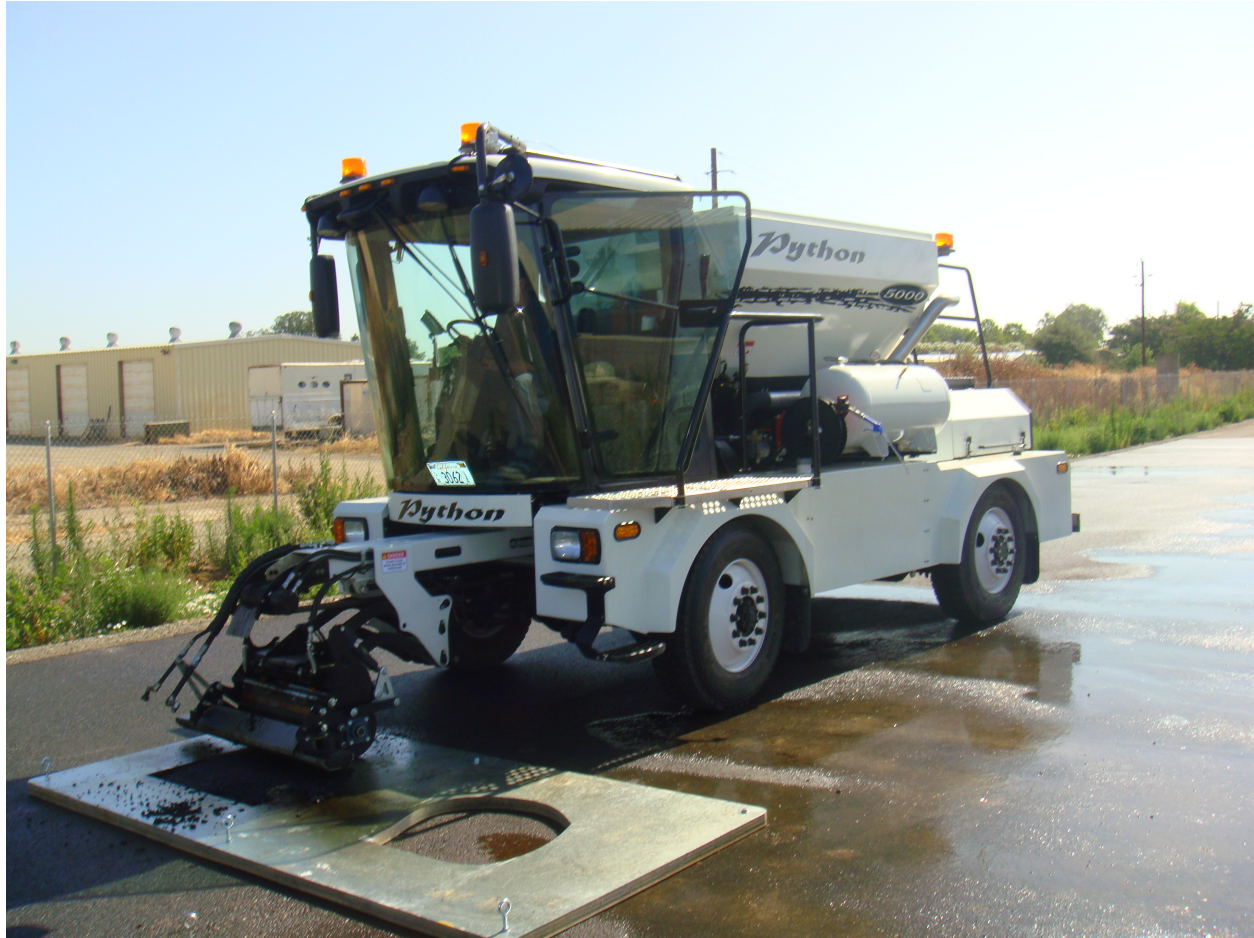
Figure 1. Python PHP 5000 Pothole Patcher During Testing at ATIRC
