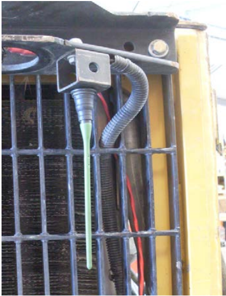
Figure 6.1: Antenna Configuration 1: Vertical, Center Offset, Close
