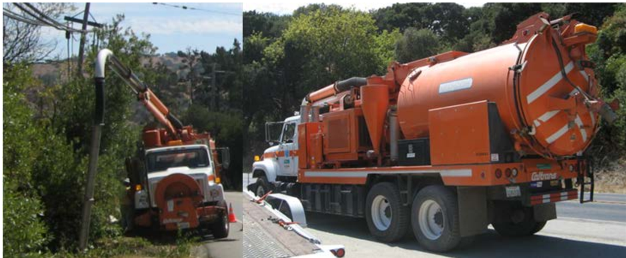
Figure 2.9: Tank system on vacuum truck with jetter system
