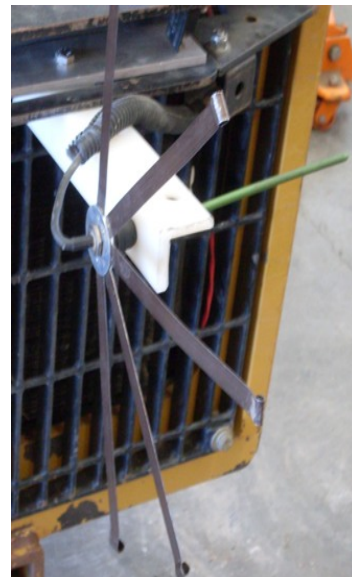
Figure 6.4: Antenna Configuration 4: Horizontal, Centered, Far, Ground Plane
