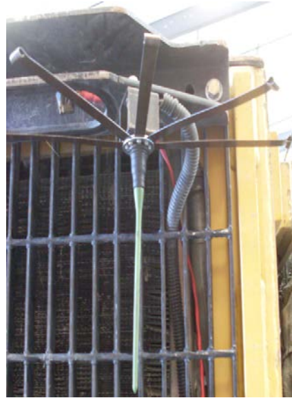
Figure 6.2: Antenna Configuration 2 : Vertical, Center Offset, Close, Ground Plane
