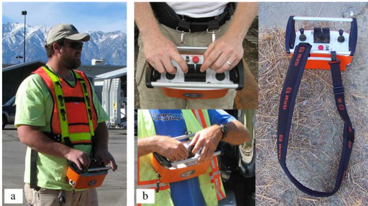
Figure 5.4: Controller carrying options: Vest (a) is much preferred over alternatives (b)
