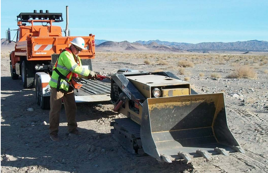
Figure 2.13: Deploying the tunnel mucker
