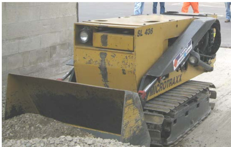
Figure 5.6: Original 3 forward facing lamps (right side hidden)
