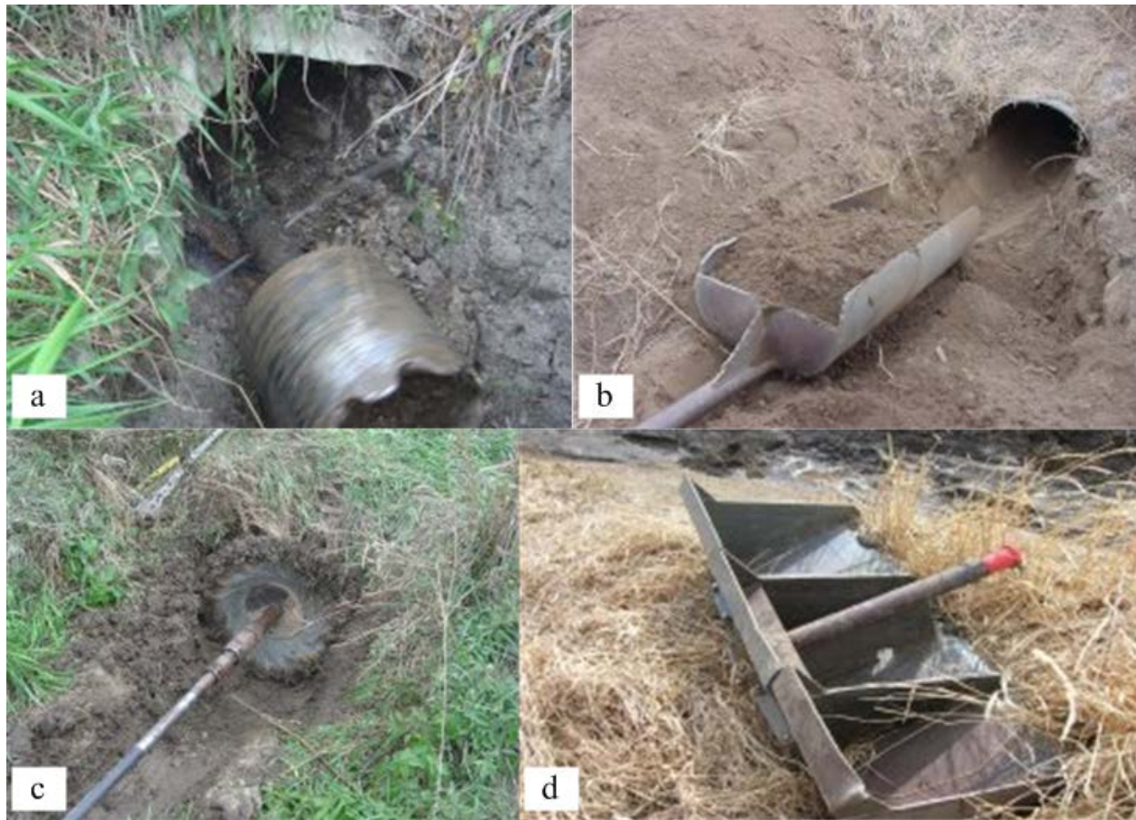
Figure 2.12: Drill attachments (a) Barrel reamer (b) Push bucket (c) Brush (d) Box tool [14]
