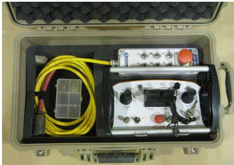
Figure 5.3: Hardened case used to carry radio components
