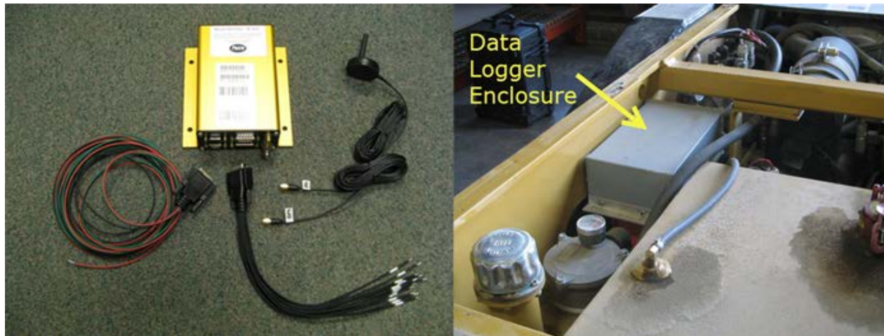
Figure 5.9: Data logger placed in custom enclosure in mucker
