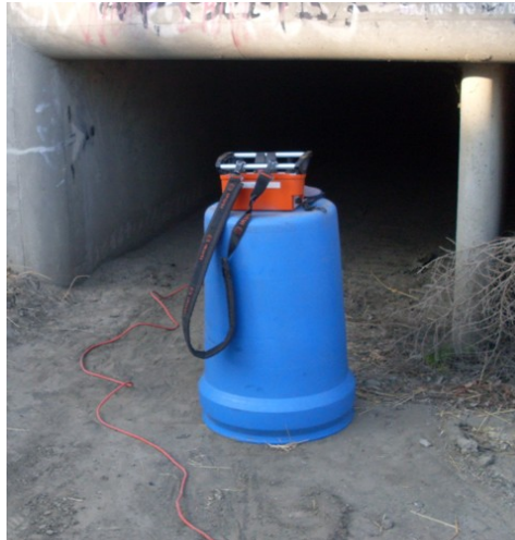
Figure 6.7: Culvert Testing transmitter configuration
