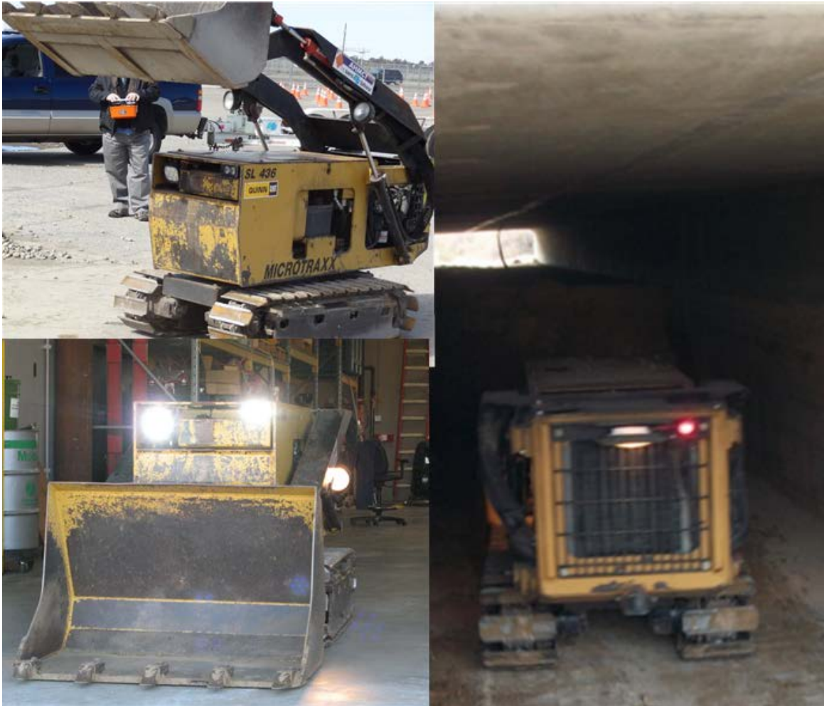
Figure 5.7: Lighting modifications: 2 LED lamps in front and red LED radio link indicator in rear
