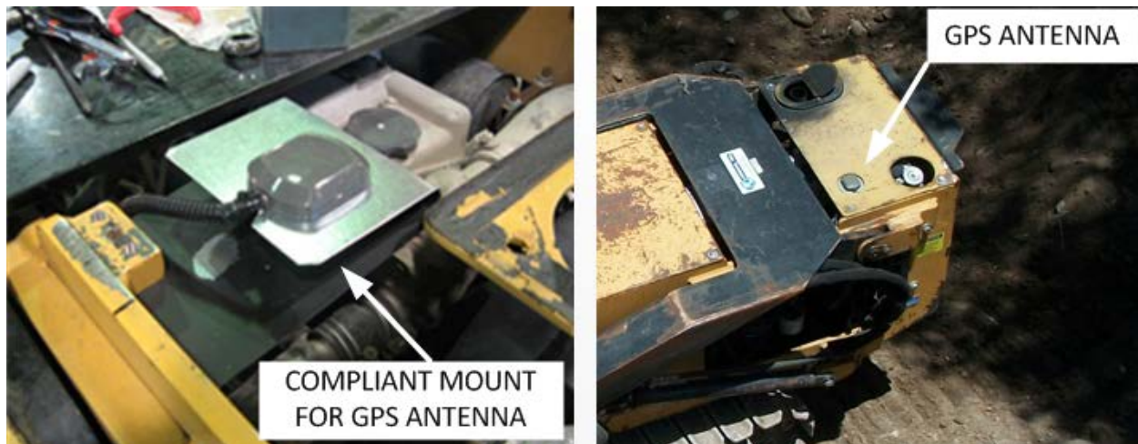
Figure 5.10: Locating the GPS Antenna
