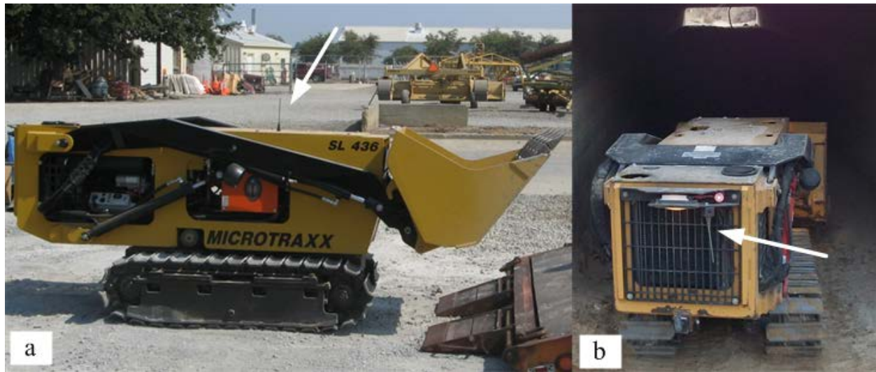
Figure 5.8: Relocation of radio control antenna from top (a) to rear (b)
