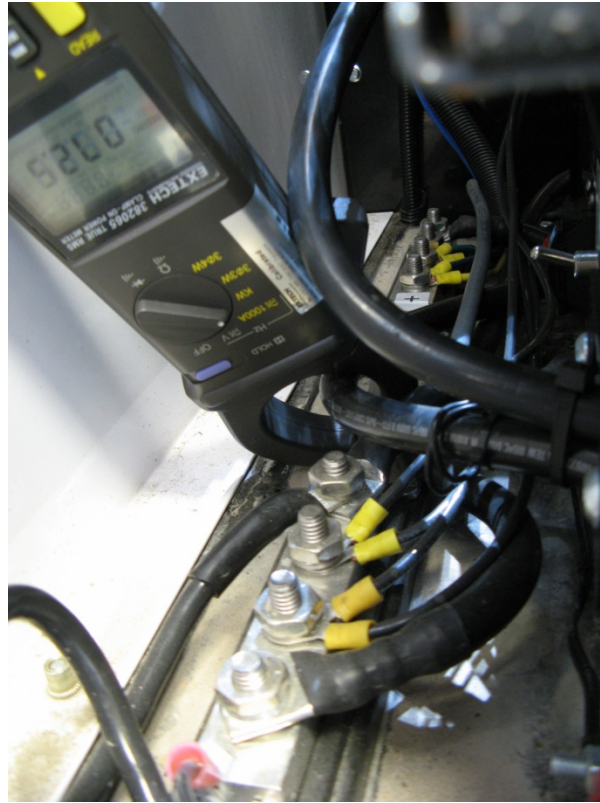
Figure 5.25: Attachment of Wattmeter to the Fuel Cell Output
