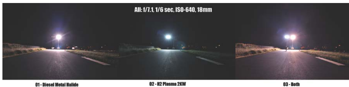
Figure 5.16: Visual Comparison of Metal Halide and Plasma Towers
