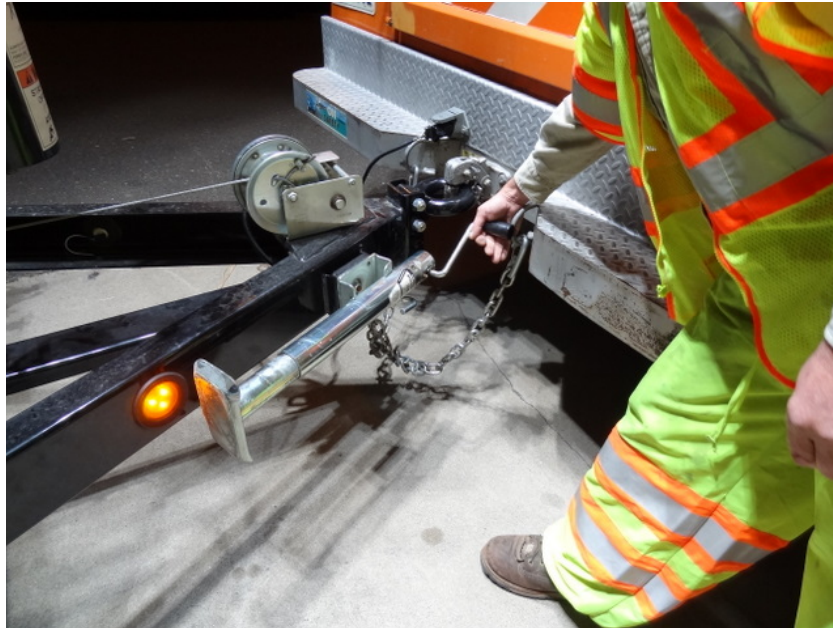
Figure 7.3: Trailer Jack Stand Should Be Moved Back, with Wheel
