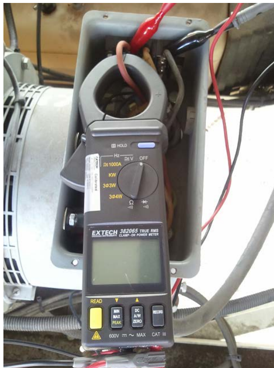
Figure 5.21: Wattmeter Measuring Current and Voltage of AC Output of Diesel Generator
