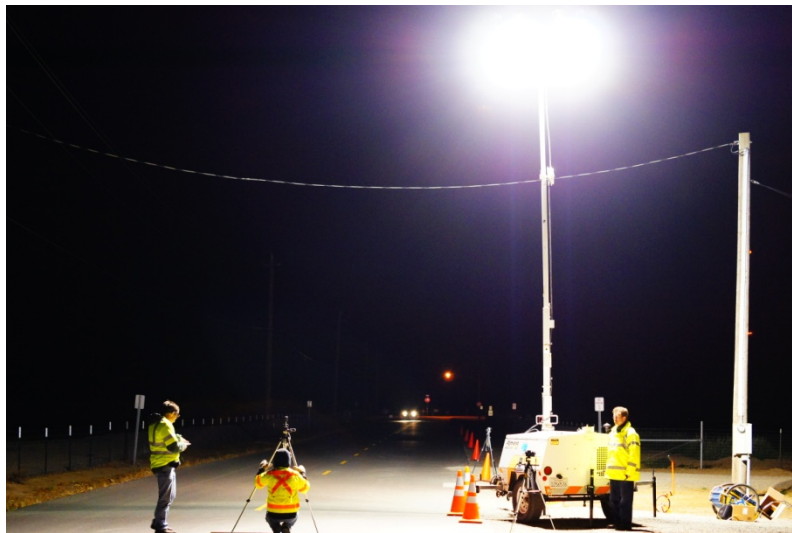
Figure 5.9: Luminance Measurement during Glare Test
