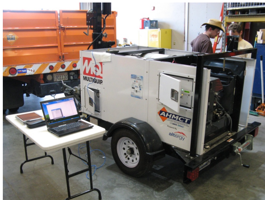
Figure 5.26: Data Logging from Internal Sensors
