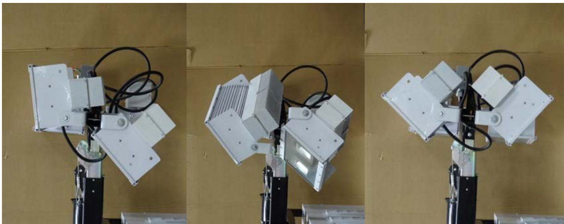
Figure 7.6: Limited Range of Motion of Plasma Luminaires
