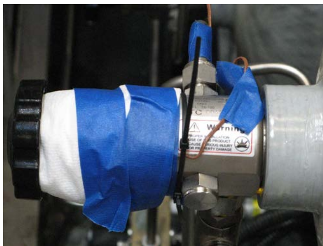
Figure 5.24: Attachment of Thermocouple to the Tank
