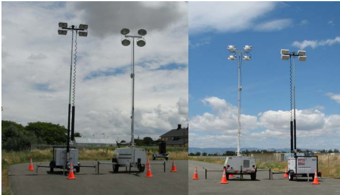
Figure 1.17: Diesel (Oval lights) and H2LT Trailers Compared in Tests
