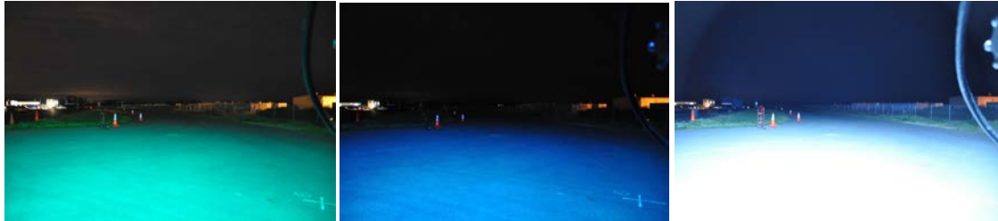
Figure 5.14: Example of Color Temperature Change during Start-up of plasma light
