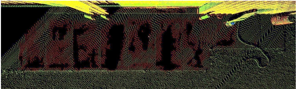
Figure C.32. Left Scanner (black area has no LiDAR return, and the red area represents the wet concrete)
