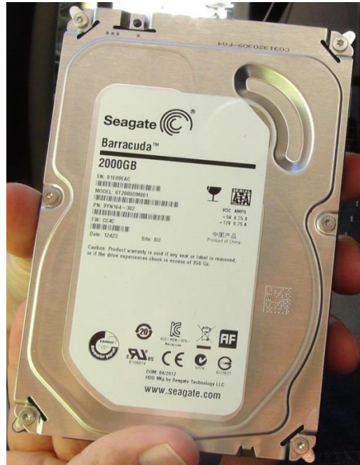
Figure A.37. MX8 data storage hard drive (Seagate Barracuda 2TB ST2000DM001)
