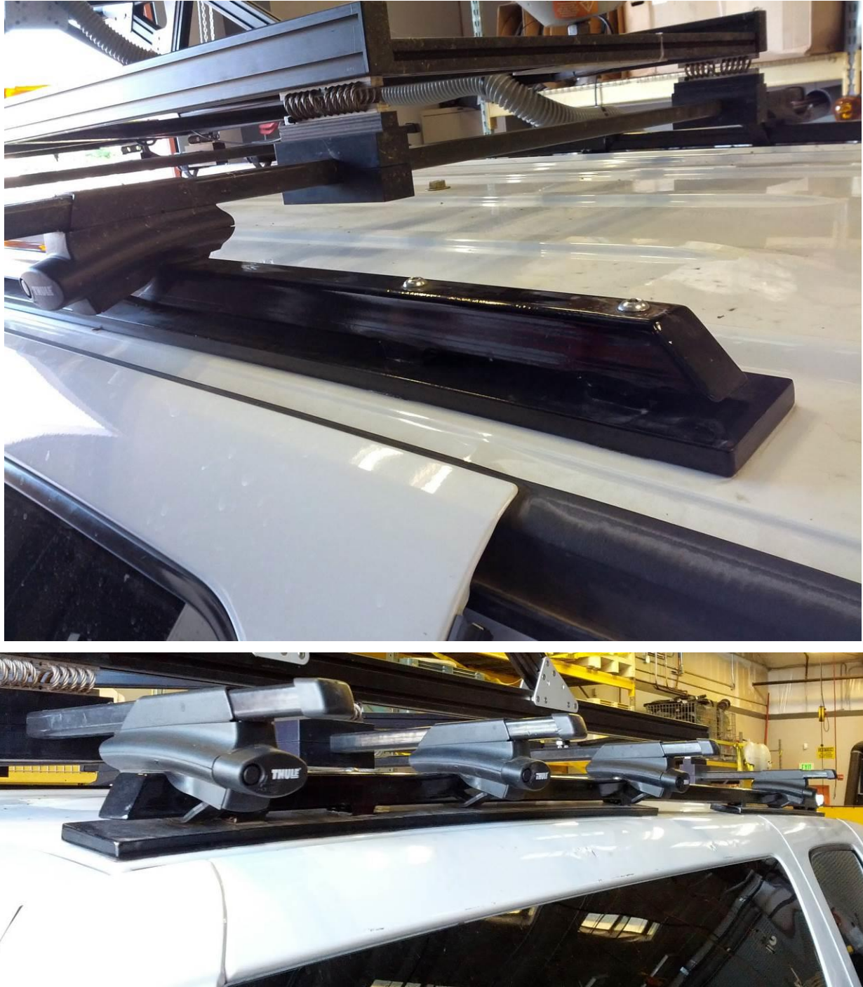
Figure 2.8. Custom roof rack made by mechanics at ESC
