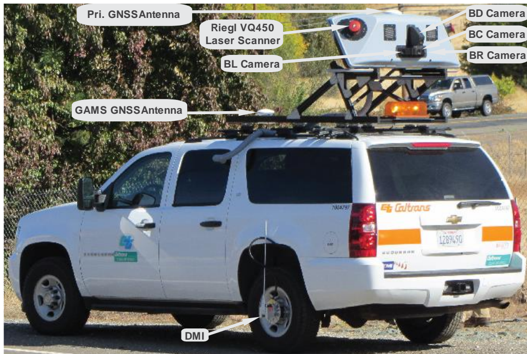
Figure A.1. Caltrans Trimble MX8 MTLS system sensor pod and DMI
