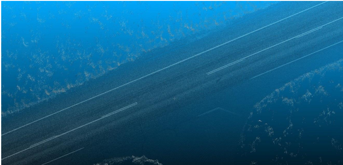
Figure 5.5. Point cloud after intensity value rescaling
