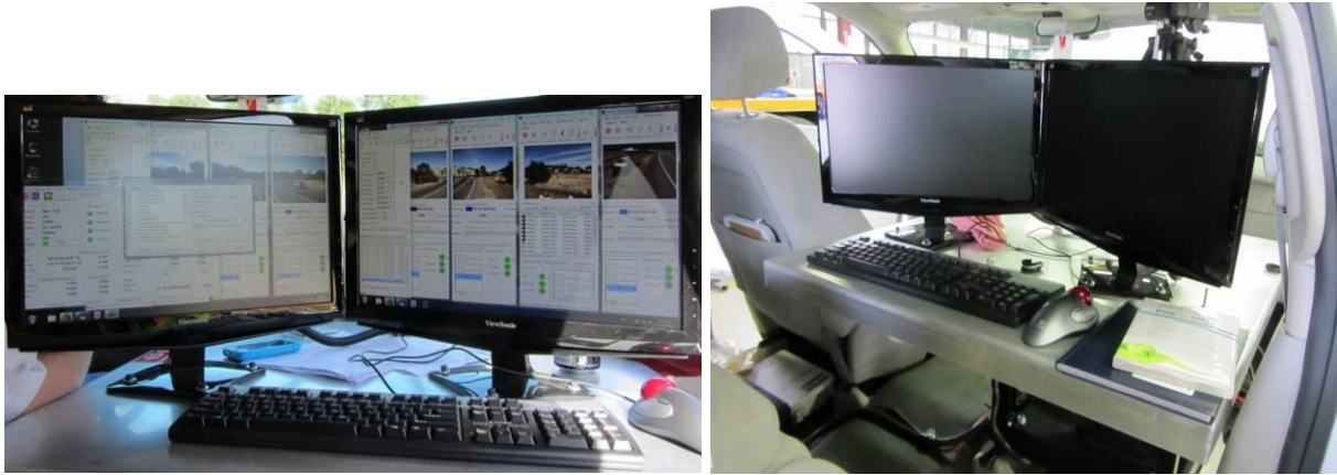
Figure 2.3. MX8 user interface (dual monitors, keyboard, and trackball) mounted next to the driver
