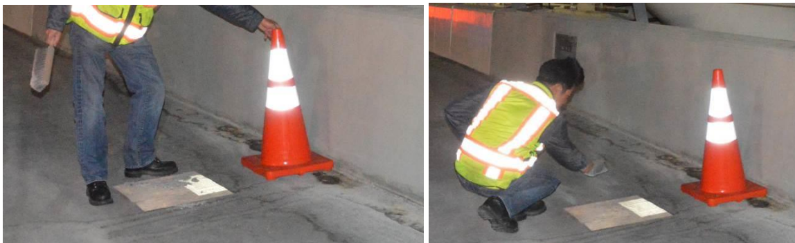
Figure 5.12. Dust and dirt accumulate on the square reflective tape target (on the left) and sweeping off dirt off target (on the right) before scanning
