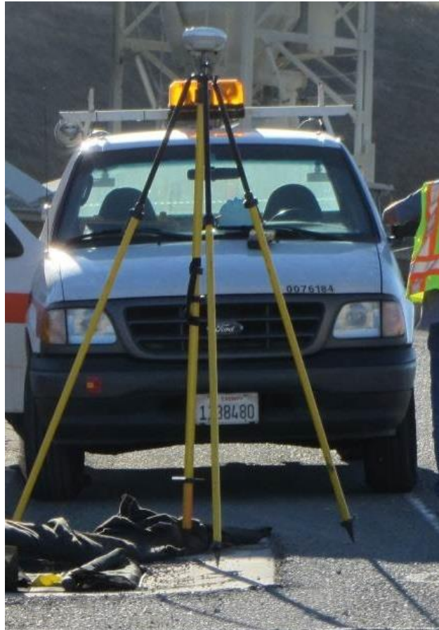
Figure 5.8. Typical GNSS base station setup over local control at the project site
