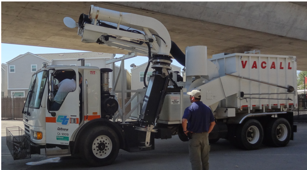
Figure 5.9 - Retracting the nozzle behind the cab
