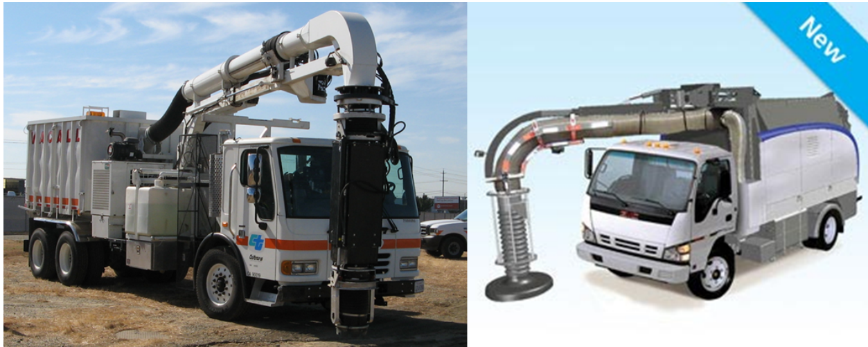
Figure 2.6 - ARDVAC (left) and Madvac LT500 (right) truck mounted telerobotic litter collector machines
