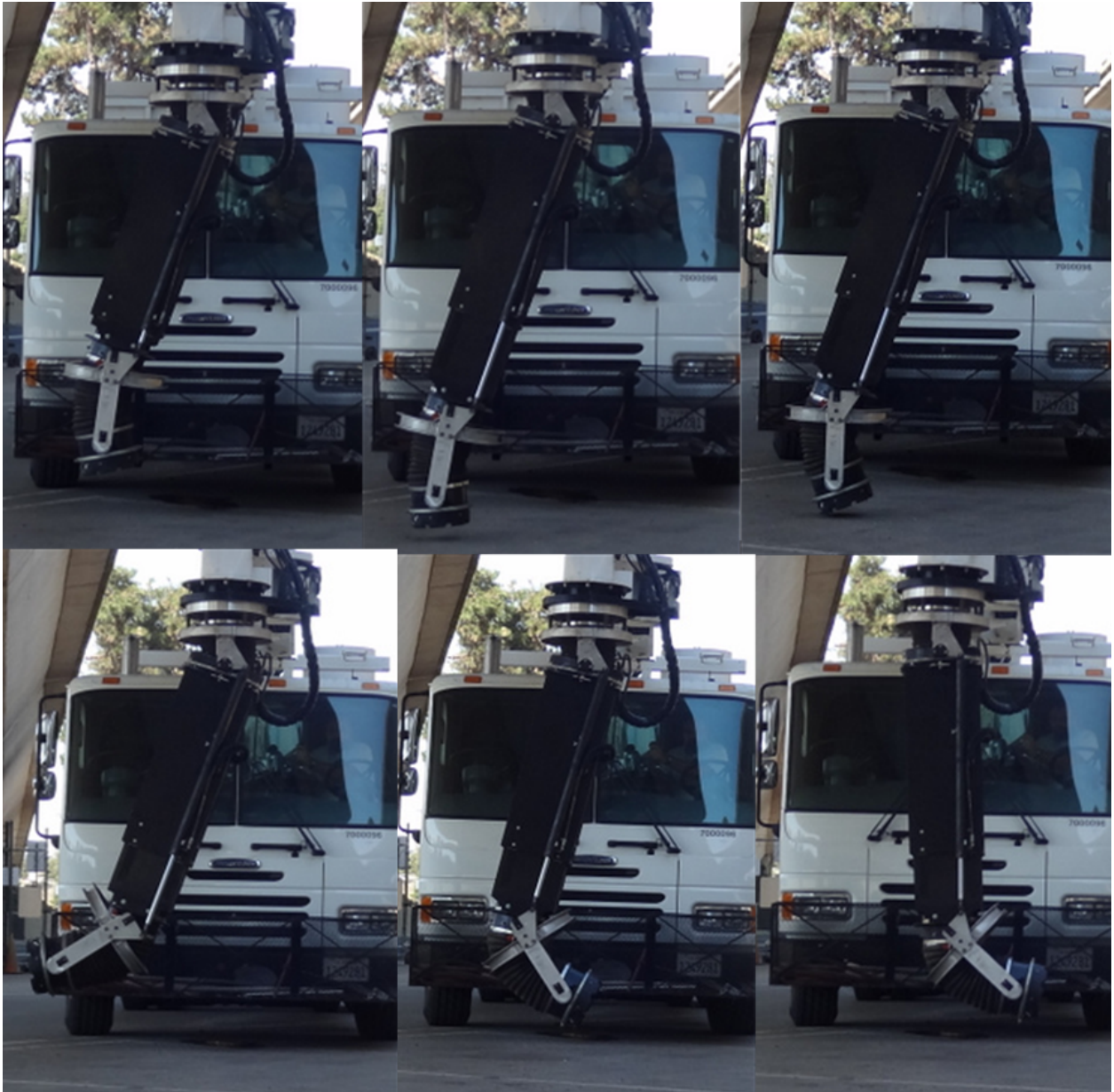
Figure 4.7 - Articulation of ARDVAC nozzle Joints 4, 5 and 6
