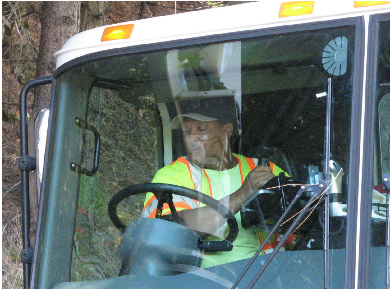
Figure 5.6 - Location of controls forces operator to rotate torso and head
