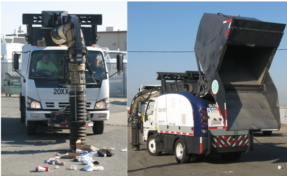
Figure 3.2 - LT500 demonstrating trash pickup and dumping
