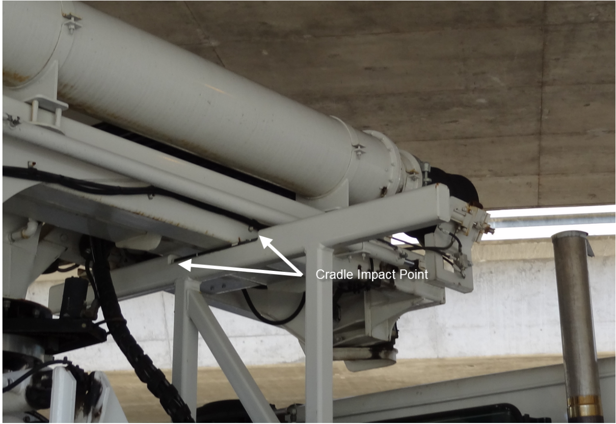
Figure 5.7 - Corners on cradle that boom impacts when moving sideways
