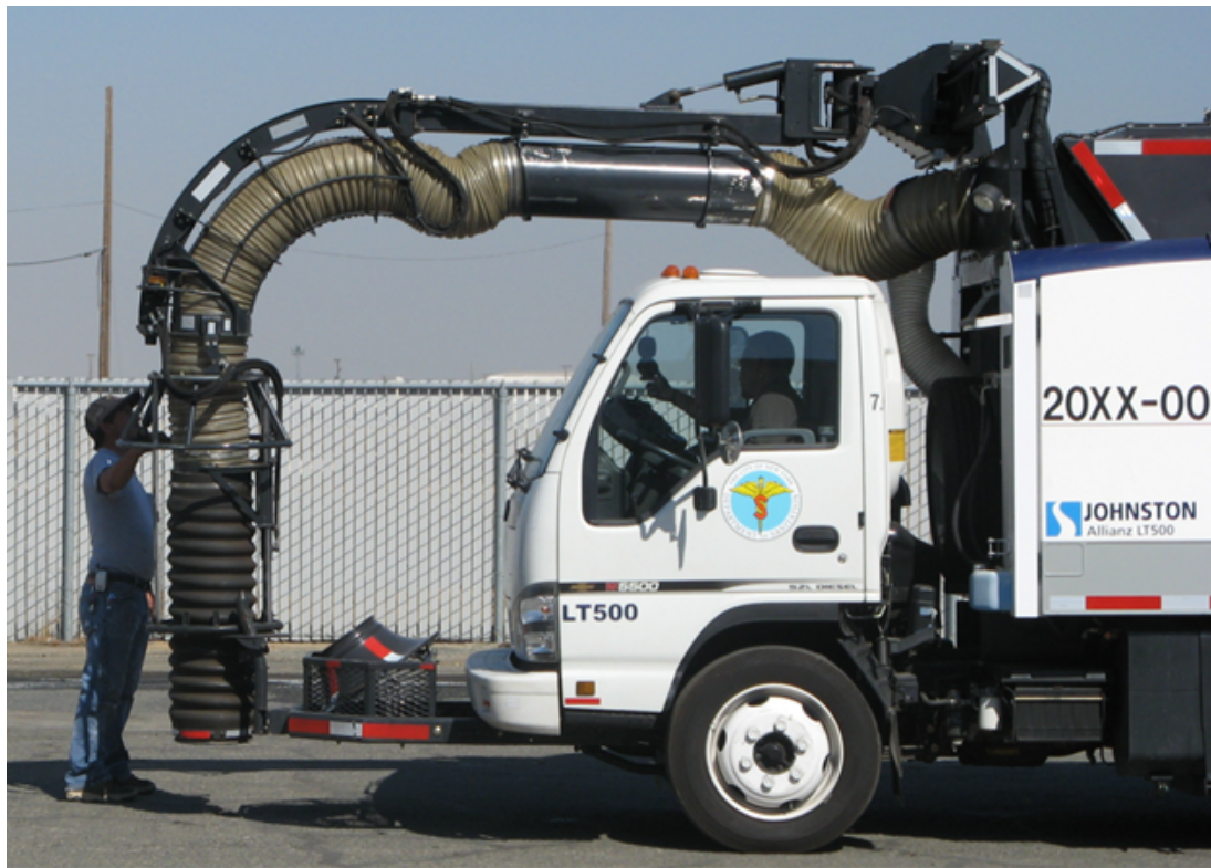
Figure 3.4 - LT500 Nozzle stowed on forward hangar
