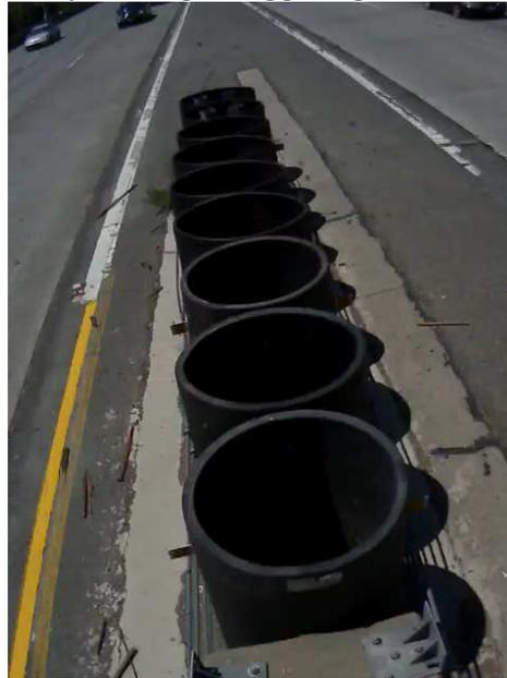
**Figure 5: Daytime view of REACT350 attenuator.**
