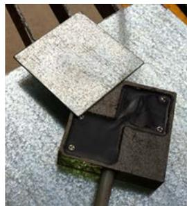
**Figure 82: Magnetic accelerometer mount with cover.**
