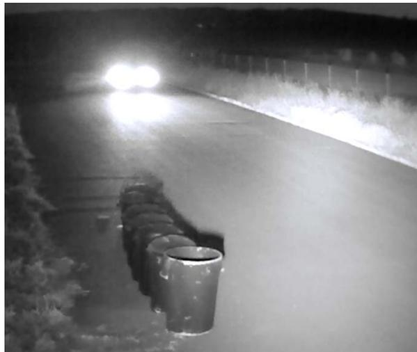
**Figure 48: Night mode with active IR lighting.**
