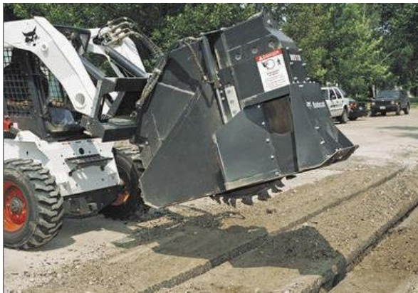
Figure 30. Bobcat Wheel Saw Attachment
