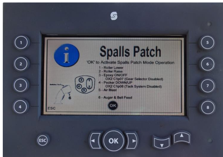
Figure 44. Spall Controls Screen
