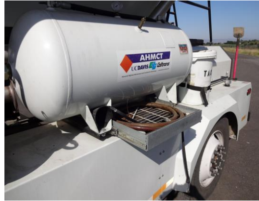
Figure 12. Python PHP Fill Hose Tray and Bucket
