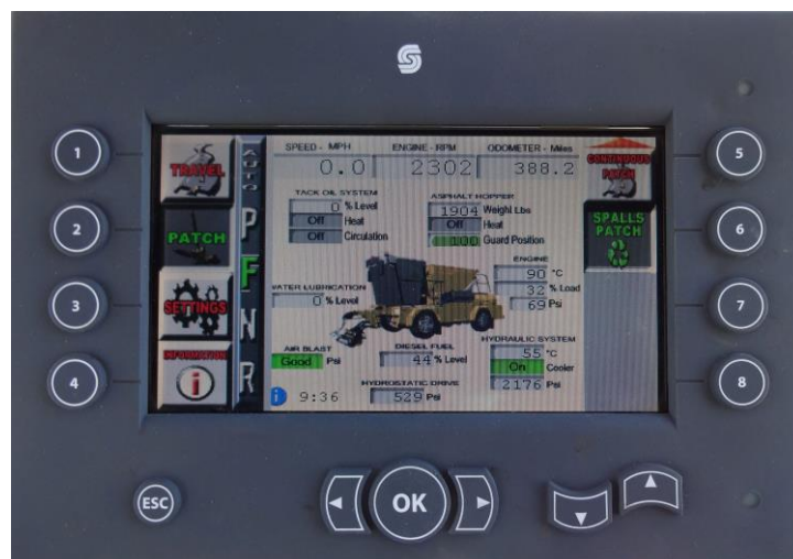
Figure 43. Spall Repair Screen
