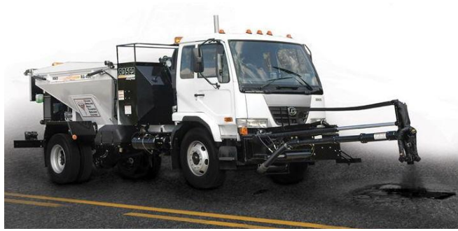
Figure 2. Rosco Spray Patch Machine
