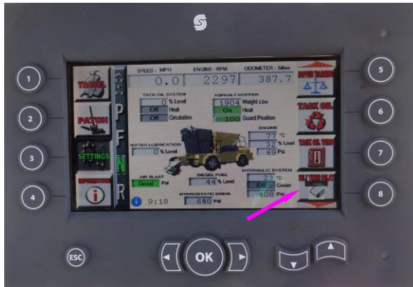
Figure 15. Settings Screen – Belt Delay
