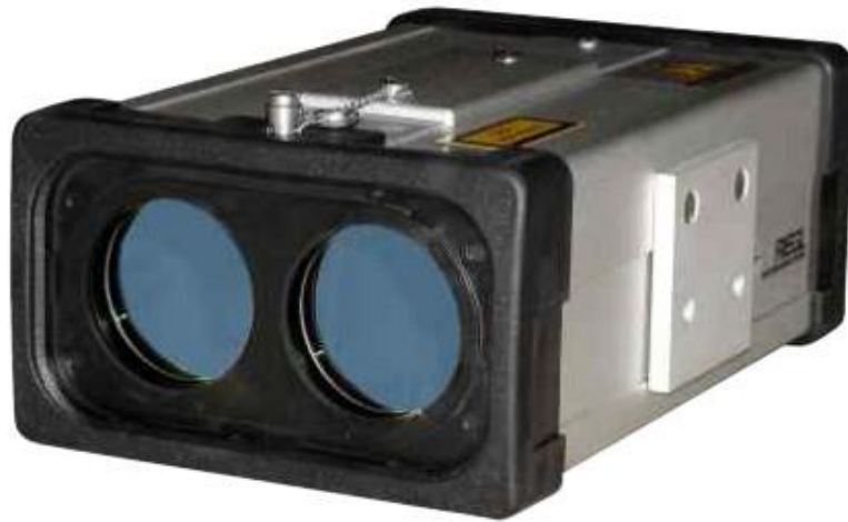
Figure 4.7: RIEGL LD90-3100 laser distance meter (courtesy of RIEGL)
