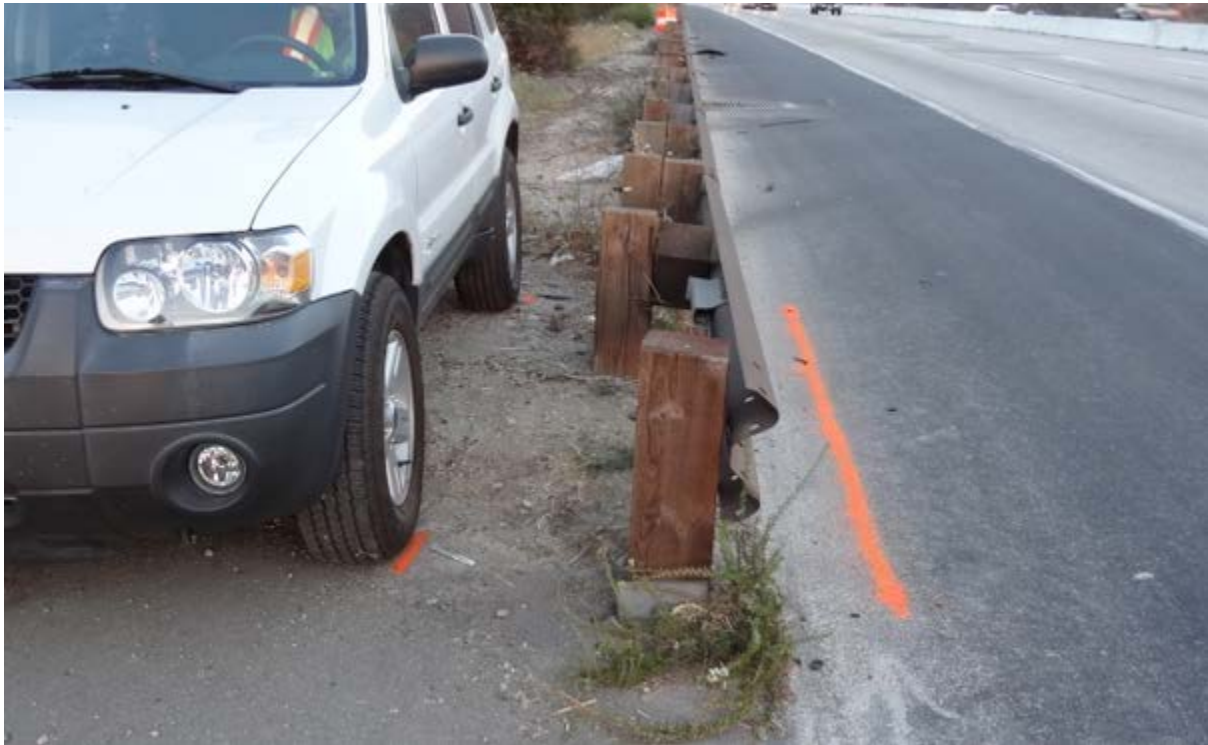
Figure 34. Alignment of a PSE System Vehicle with Respect of the Road Edge Using a Line Parallel to the Fog Line.
