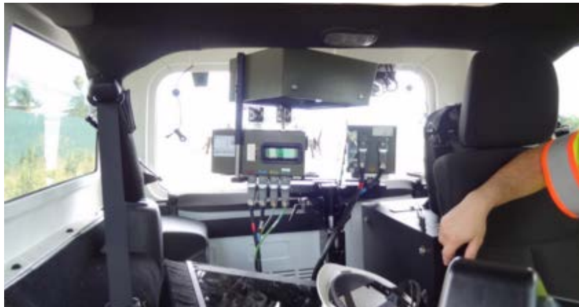
Figure 35. Example of PSE System Components.
