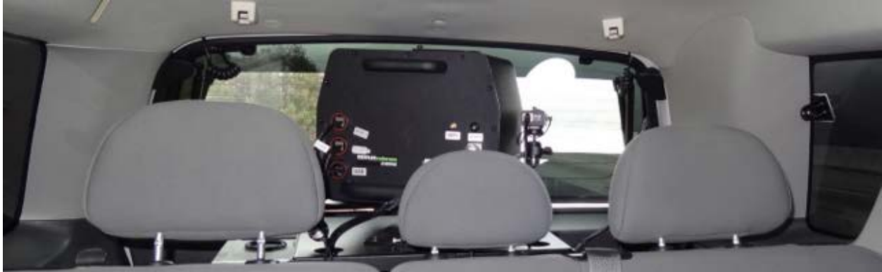
Figure 37. View of a PSE System From Behind Rear Seat of a Small SUV with the Operator Facing Forward.
