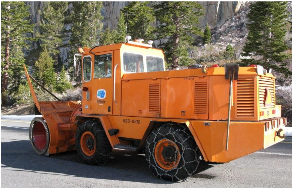
Figure 3.5: Caltrans rotary snow blower with GPS antenna bar
