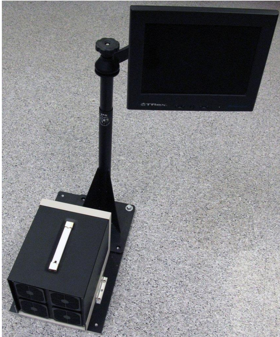
Figure 3.3: Liquid Crystal Display (LCD) and system box containing computer and GPS receivers
