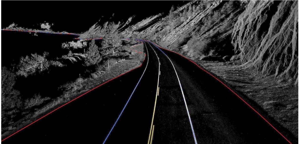
Figure 4.8: Point cloud with extracted feature lines overlaid in Cyclone. The red, blue, and yellow lines denote the edge of pavement, fog line, and centerline, respectively.
