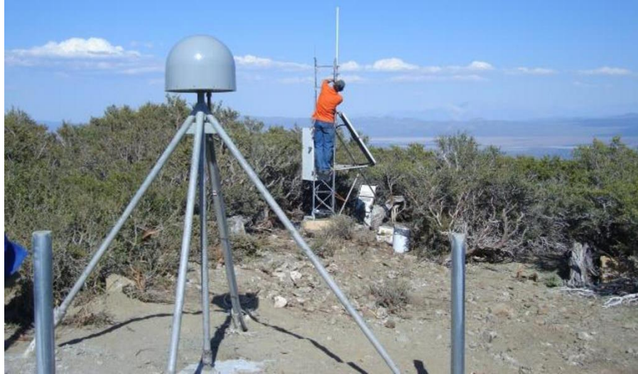
Figure 4.3: CORS station P636 setup (Image from http://www.ngs.noaa.gov/cgi-cors/corsage.prl?site=P636 )
