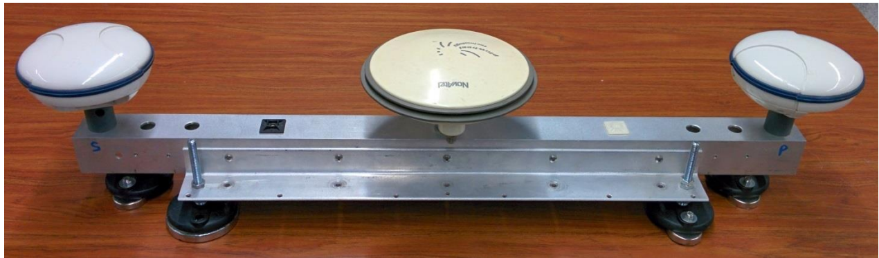
Figure 3.4: GPS antenna bar with magnetic mount
