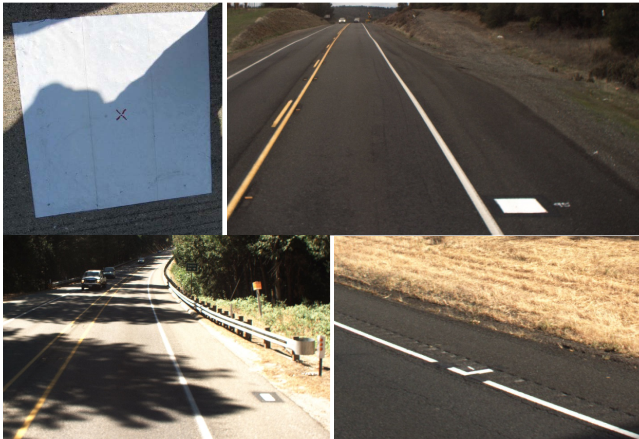
Figure 5. Sample ground control targets located on the road shoulder.
