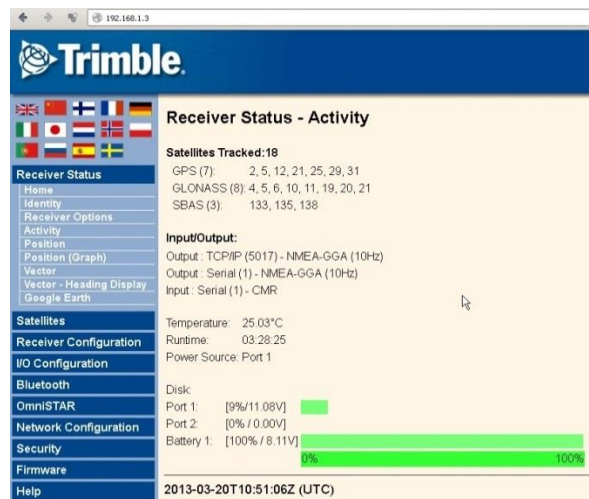
Figure 4.7: Trimble GNSS receiver web user interface showing power supply voltage at 11.08 v when heater is running
