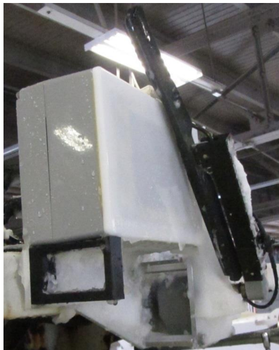
Figure 4.13: Third-generation wiper design (wiper motor mounted on bottom) with heated wiper blade
