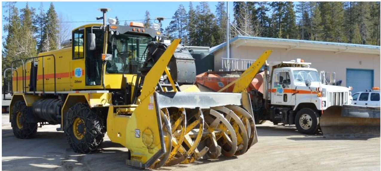
Figure 2.1: Snowplow DAS installed on Caltrans snow blower (left, yellow) and snowplow (right, white)
