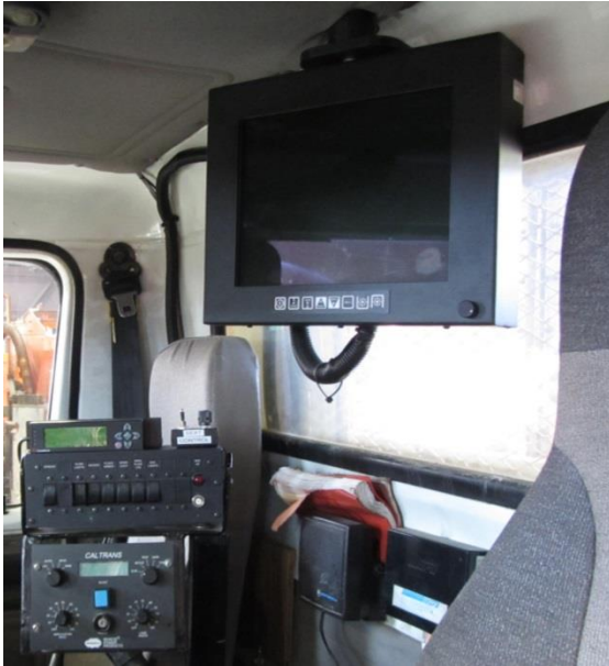
Figure 2.2: DAS user interface and LCD imager display on snowplow
