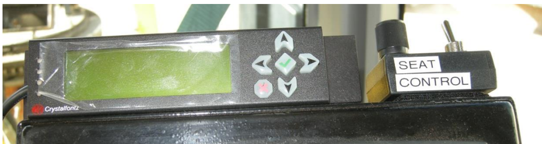
Figure B.5: DAS user interface. The Crystalfontz LCD touchpad is on the left, and the seat controller is on the right.
