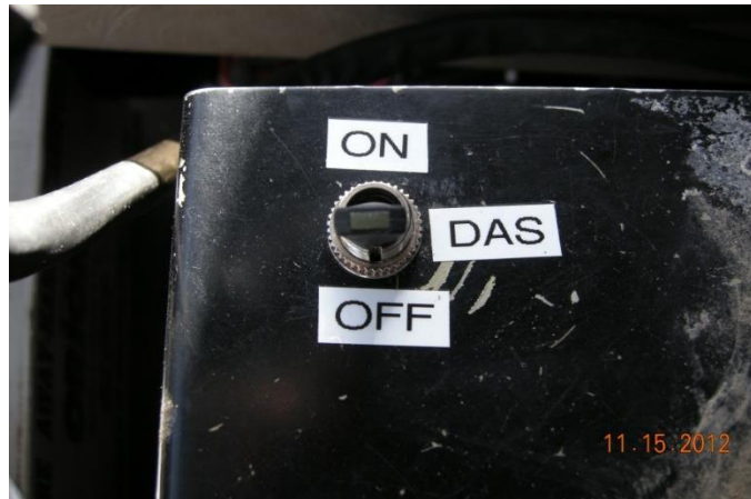
Figure B.4: Driver Assist System (DAS) ON/OFF switch for plow 0530506 located beneath the Muncie spreader controls
