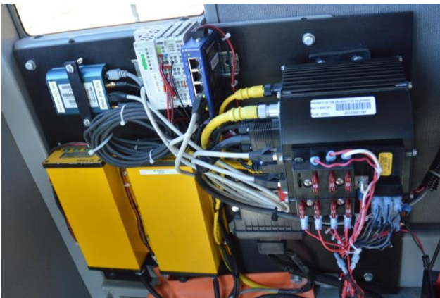
Figure 2.12: DAS equipment mounted next to the operator's seat in the snow blower
