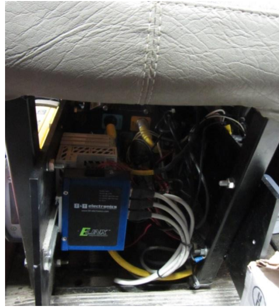
Figure 2.3: DAS installed under the passenger seat on snowplow
