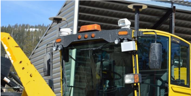
Figure 2.8: DAS exterior components (radar & GNSS antenna) on snow blower
