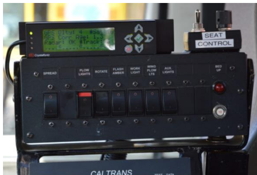
Figure 2.6: DAS user interface and vibration seat control on snowplow
