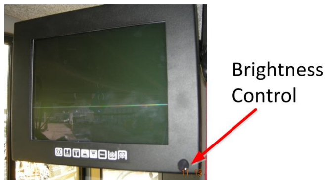
Figure B.3: Brightness control for HUD image source
