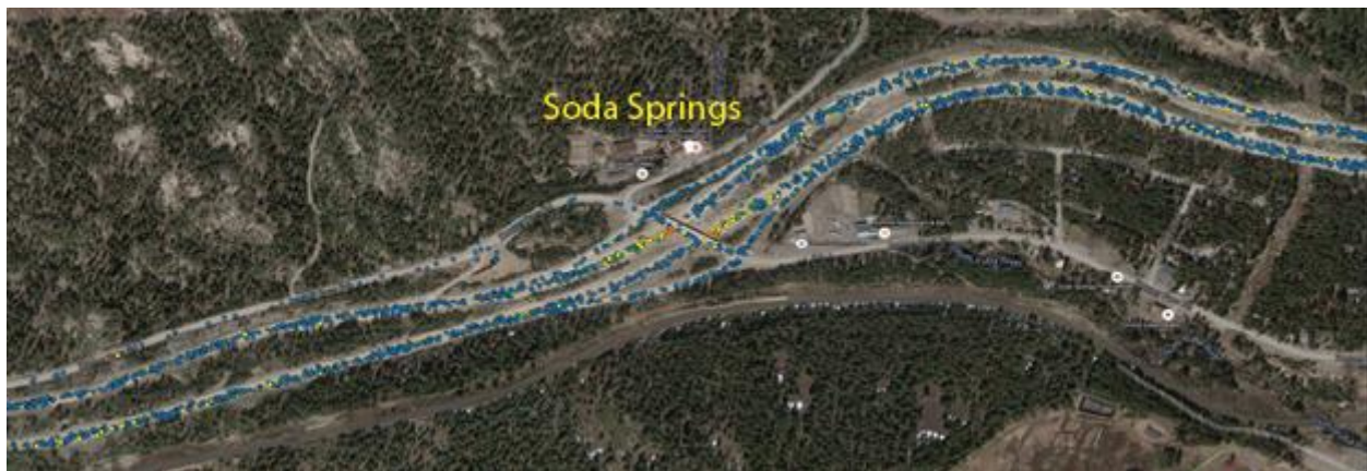
Figure 5.9: GNSS RTK solution status on I-80 at Soda Spring overlaid on a Google hybrid map
