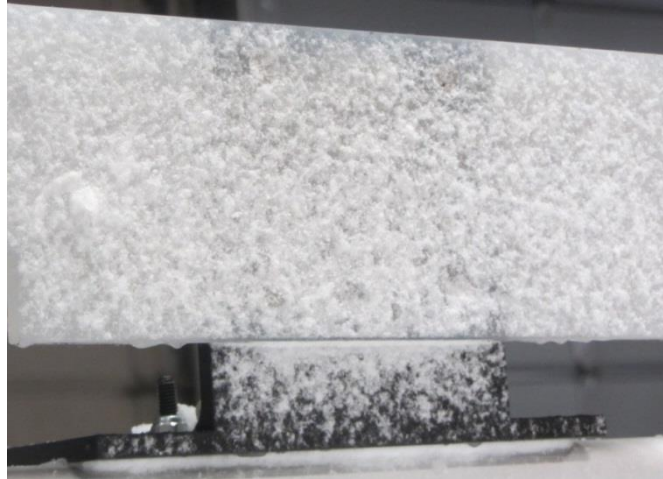
Figure 4.9: Icing on polycarbonate plastic coated with Rust-Oleum NeverWet after driving in a snow storm
