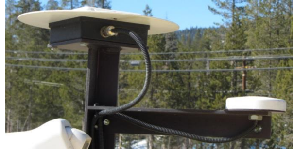
Figure 2.9: GNSS antenna & modem antenna mounted on snow blower
