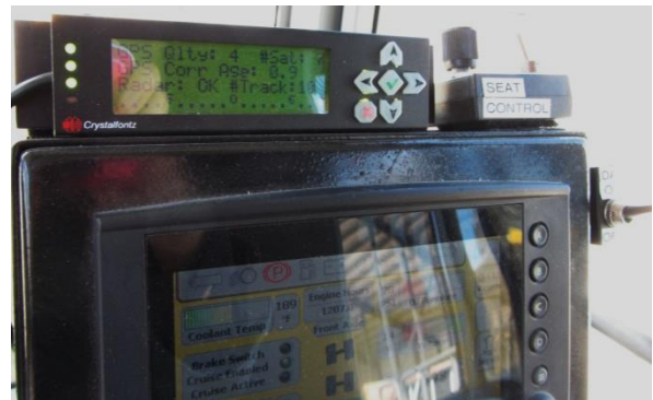
Figure 2.11: Driver's view looking through the combiner in the snow blower
