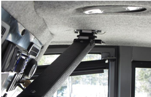
Figure 2.10: DAS HUD combiner mount in the snow blower
