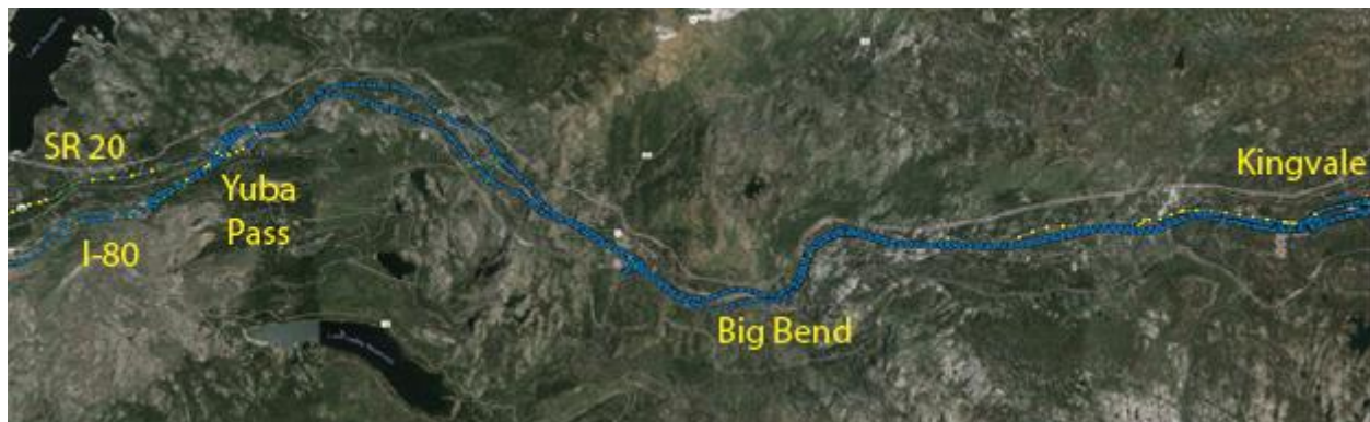
Figure 5.6: GNSS RTK solution status on I-80 from SR 20 intersection to Kingvale overlaid on a Google hybrid map
