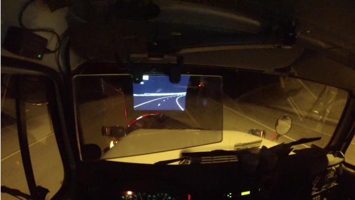
Figure 2.14: DAS viewed from behind driver's seat in a snowplow operating at night. The lane lines and road features are overlaid on the road using the HUD.
