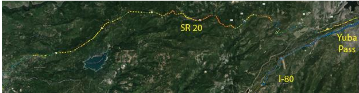
Figure 5.7: GNSS RTK solution status on SR 20 overlaid on Google hybrid map
