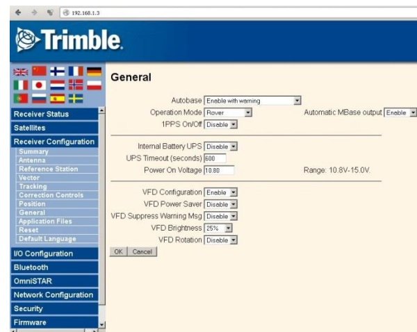
Figure 4.8: Trimble GNSS receiver web user interface showing power on voltage set to 10.8 v
