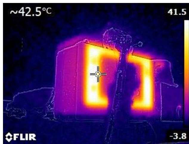
Figure 4.11: Thermal image of the first-generation wiper / heated enclosure system
