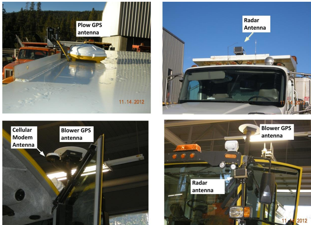
Figure B.1: System components mounted on the outside of the vehicles
