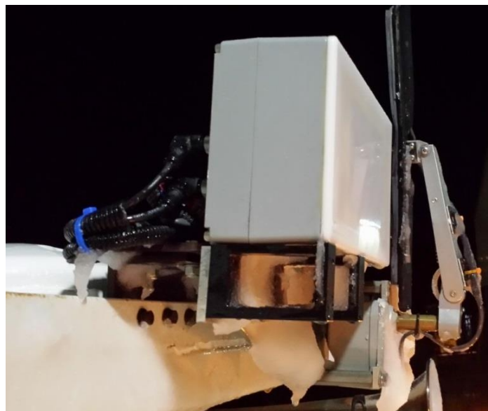
Figure 4.15: Final wiper design with heated wiper blade. This design passed operational testing. Snow accumulated in areas surrounding the radar, but not on the fascia.
