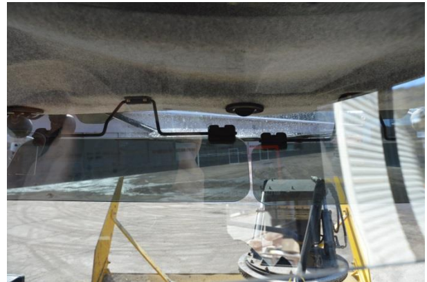
Figure 2.11: Driver's view looking through the combiner in the snow blower
