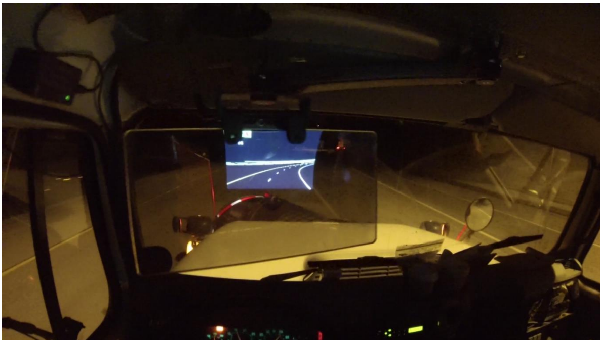
Figure 1.5: DAS viewed from behind driver's seat in a snowplow operating at night. The lane lines and road features are overlaid on the road using the HUD.
