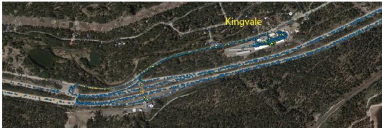
Figure 5.8: GNSS RTK solution status on I-80 at Kingvale area overlaid on a Google hybrid map
