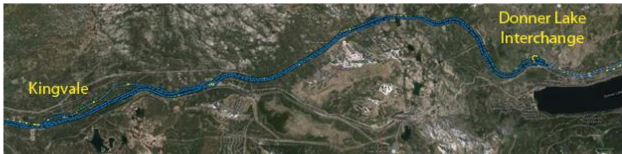
Figure 5.5: GNSS RTK solution status on I-80 from Kingvale to DLI overlaid on a Google hybrid map
