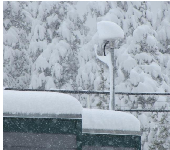
Figure 2.17: GNSS base station antenna functioning under heavy snow cover
