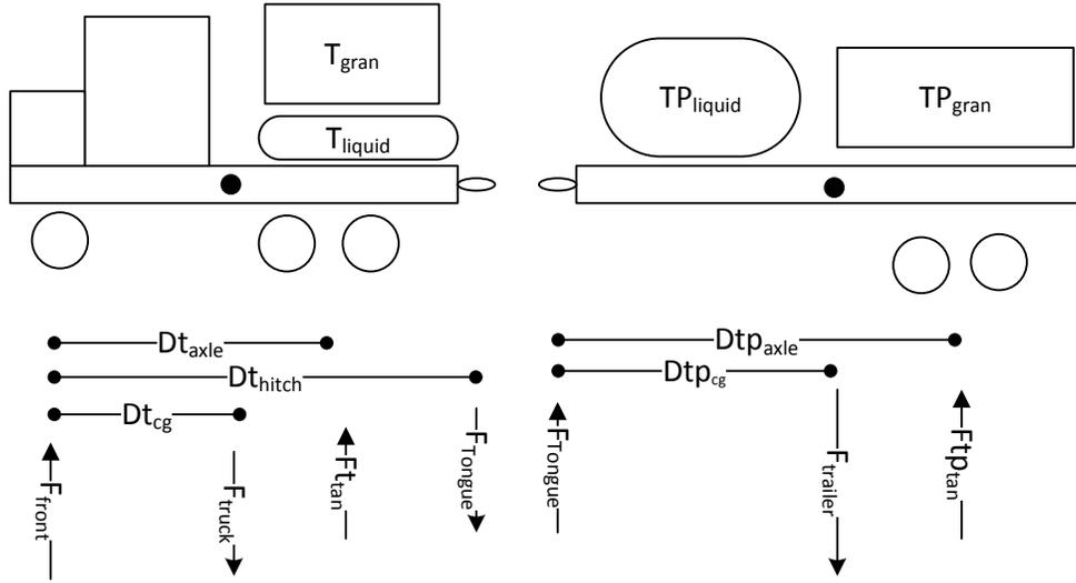
**Figure 83. Free body diagram of TowPlow2**
