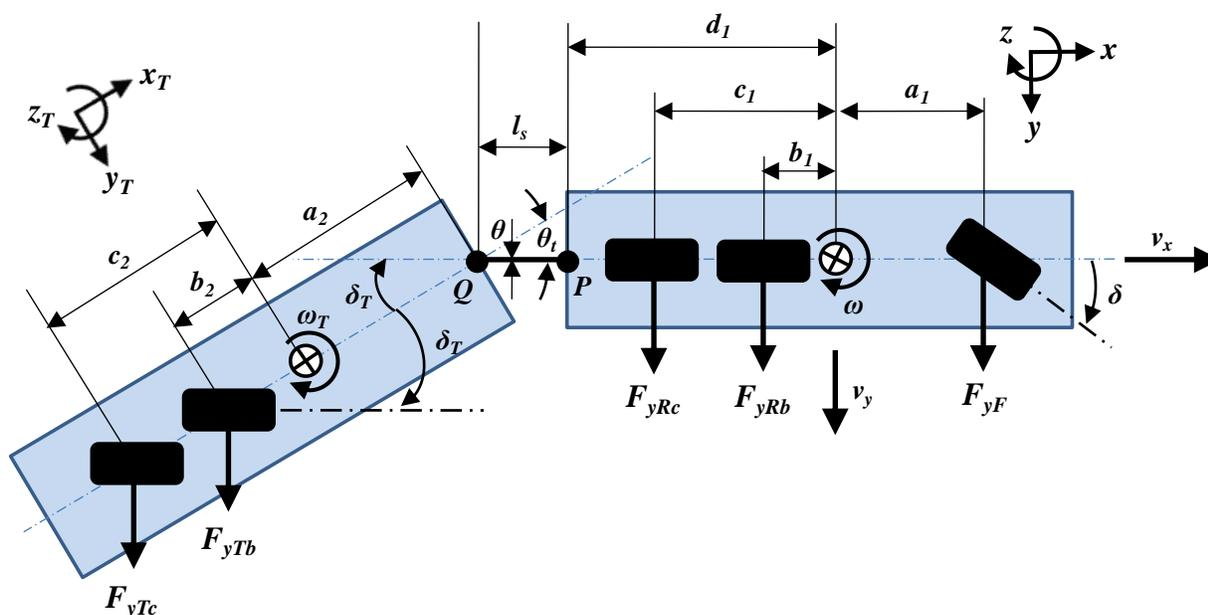
Figure 27. Linear planar TowPlow model and parameters
