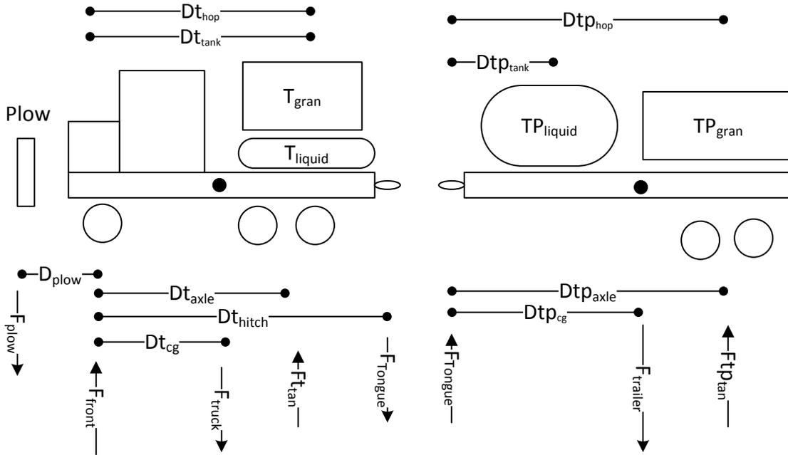
Figure 84. Free body diagram of TowPlow2
