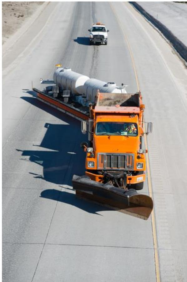
**Figure 1. A TowPlow system in its deployed configuration**
