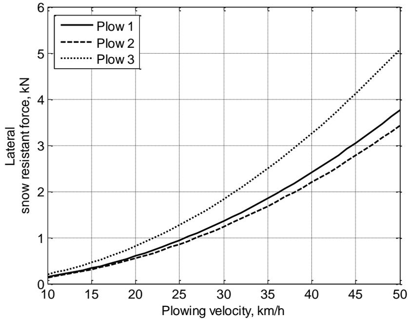
Figure 59. Lateral snow resistant forces of the plows
