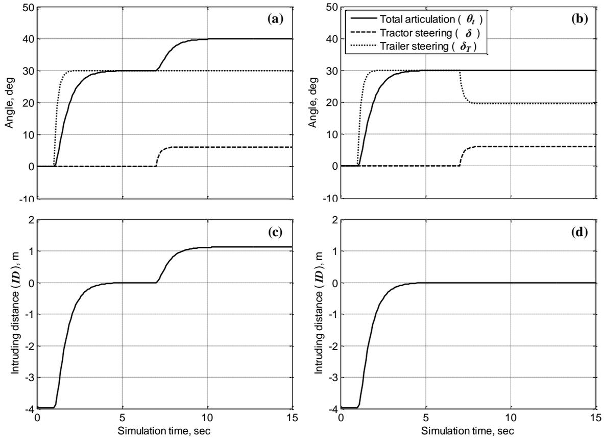
**Figure 26. Simulation results of the constant radius turning: (a) angles without trailer corrective steering, (b) angles with trailer corrective steering, (c) intruding distance without trailer corrective steering, (d) intruding distance with trailer corrective steering**
