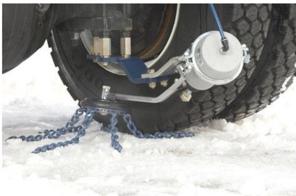
**Figure 3. Onspot chain system [www.onspot.com]**
