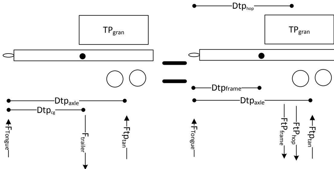
Figure 85. TowPlow2 trailer free body diagrams
