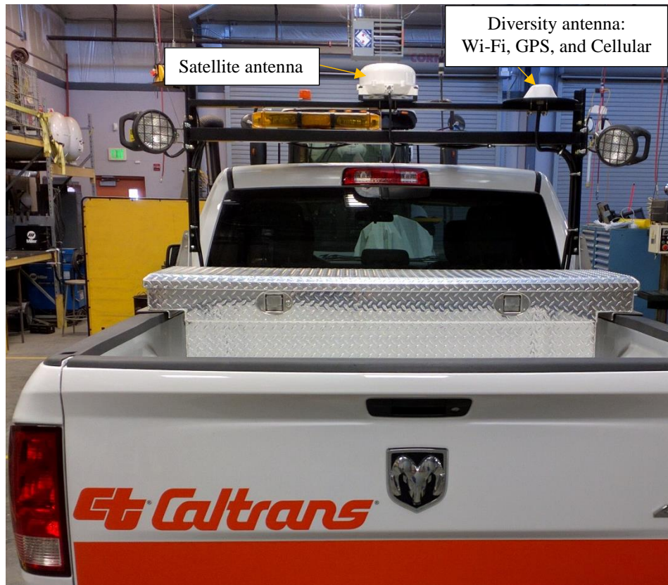
Figure 5.28: Responder system diversity antenna on right side of the vehicle light bar. This incorporates antennas for Wi-Fi, cellular, and GPS.
