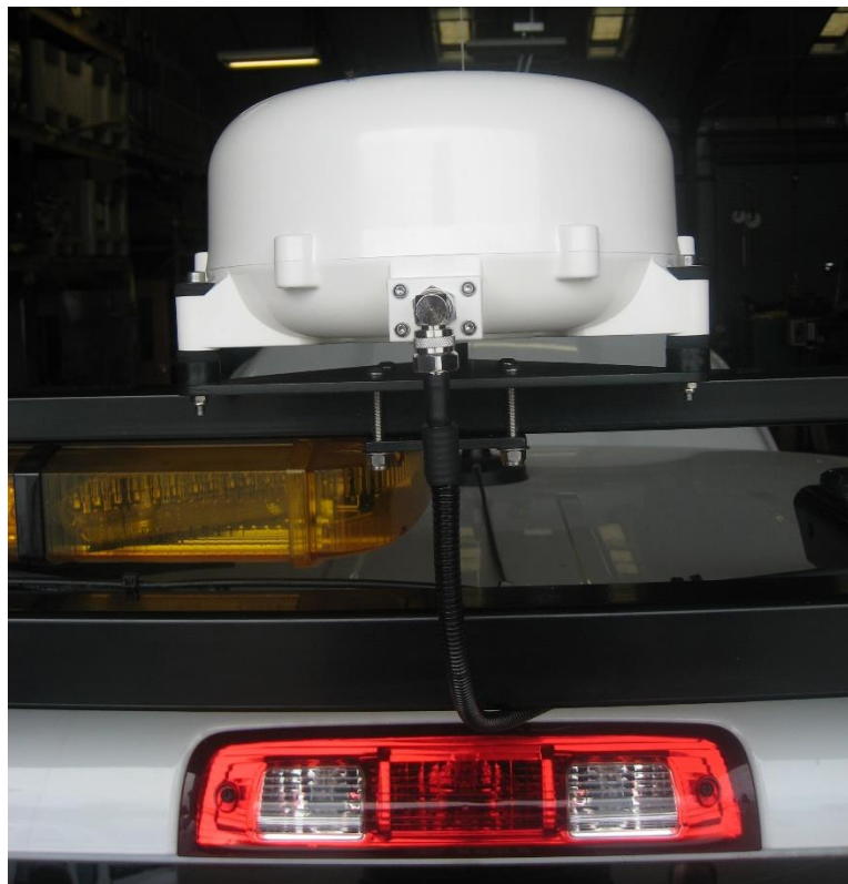
Figure 5.26: Satellite antenna mounted on vehicle light bar
