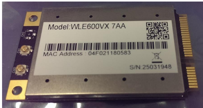
Figure 5.29: Responder system Wi-Fi card installed inside the Responder computer system (Logic Supply Nuvo-3100VTC embedded computer)
