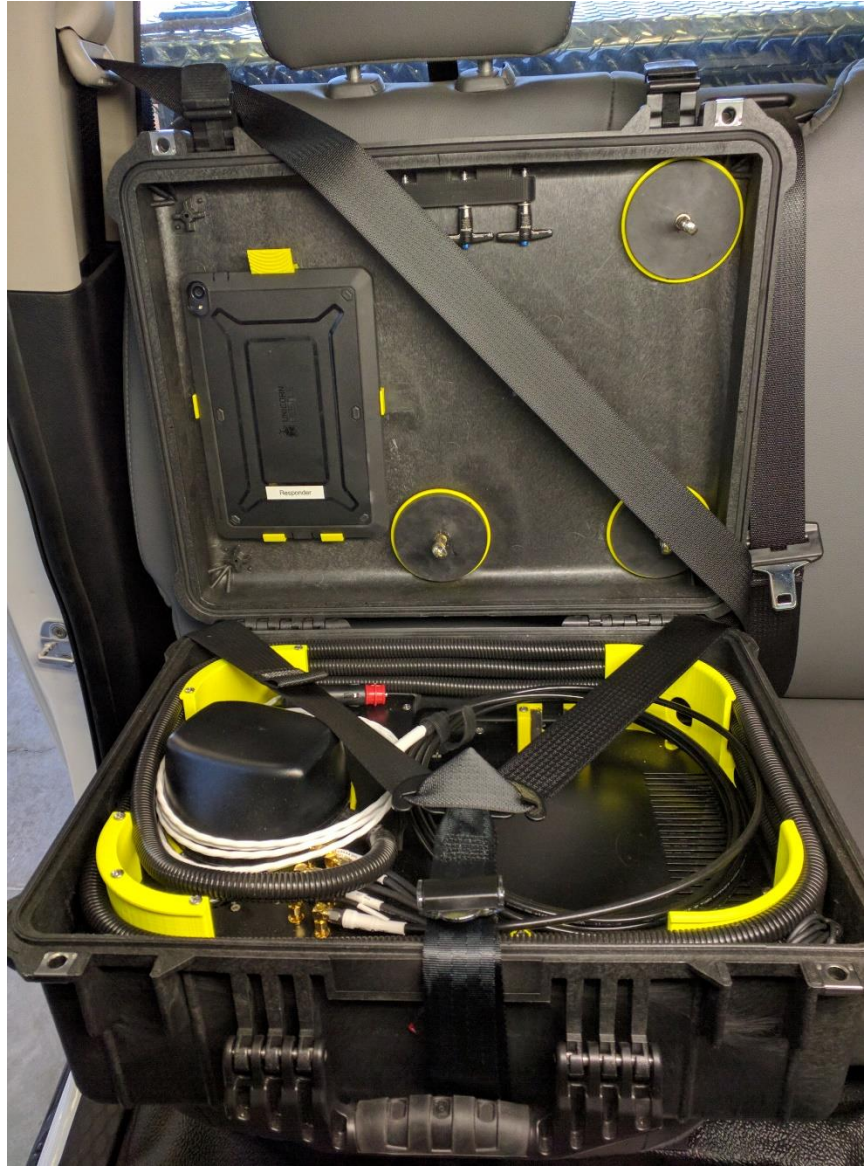
Figure 5.32: Tentative method for restraining the Portable Responder system
