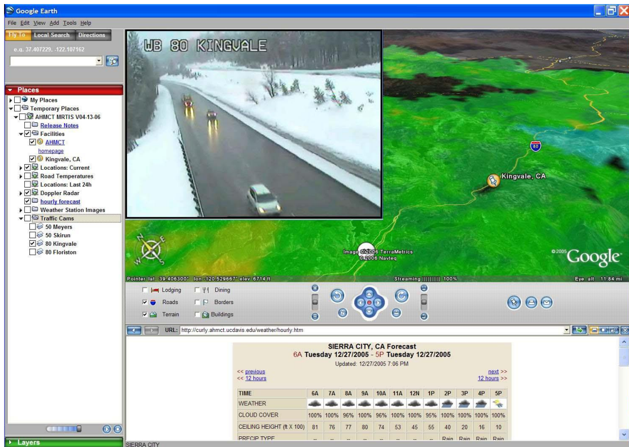
Figure 2.6: Example snow fighter information system in-vehicle display integrating radar, weather forecasts, terrain, vehicle locations, traffic, and road surface condition. This is a prototype display from Phase 1 research[18].
