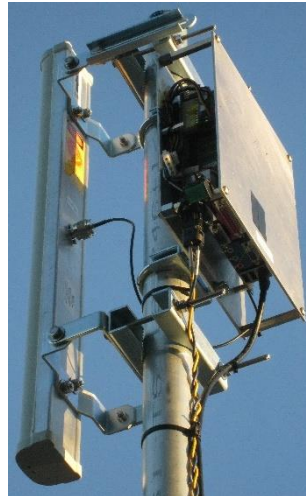
Figure 3.5: AHMCT 5.8 GHz point-to-point communication experimental setup
