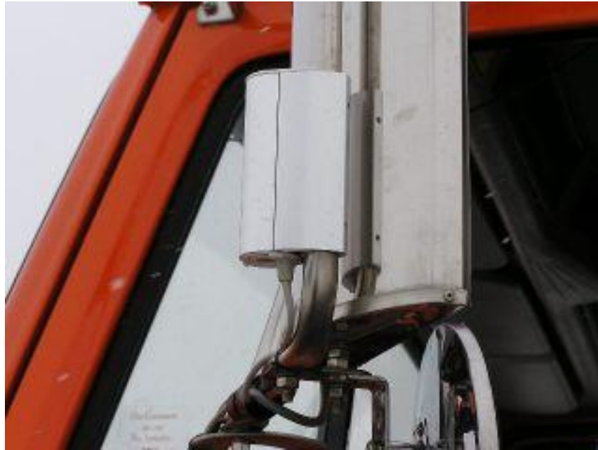
Figure 5.4: RoadWatch air and pavement temperature sensor
