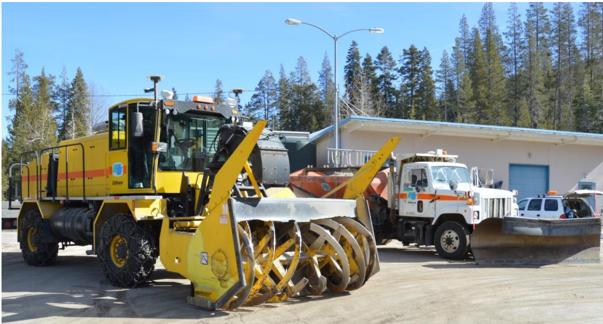
Figure 1.1: Snowplow Driver Assistance System installed on Caltrans snow blower (yellow) and snowplow (white)
