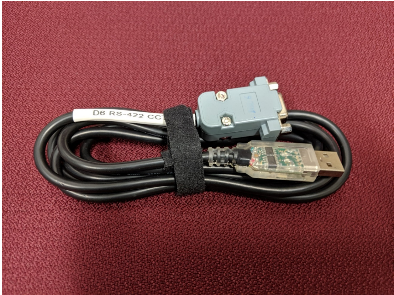
Figure 5.11: HHDC kit USB serial RS-422 to D6 CCTV DE-9 connector
