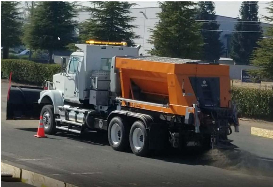
**Figure 8: Epoke SH 4900 spreader, truck ID 7010966**
