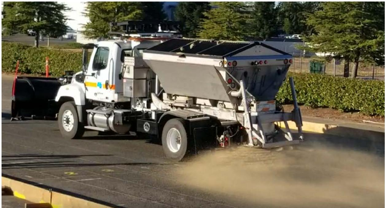
**Figure 6: Vbody Spreader - Henderson Model FSH, truck ID 7008268**
