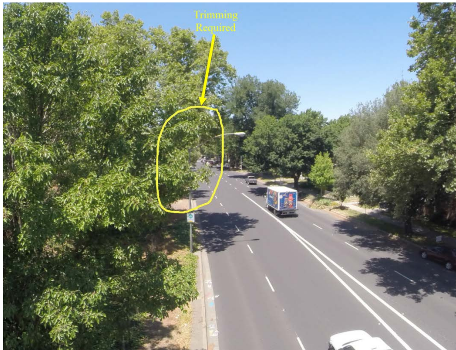
Figure 3.2: Example of tree trimming required to provide better camera FOV (US 50 WB 10 th St exit)
