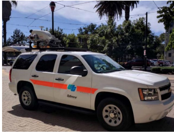
Figure 2.18 Caltrans Mobile Terrestrial Laser Scanning (MTLS) vehicle
