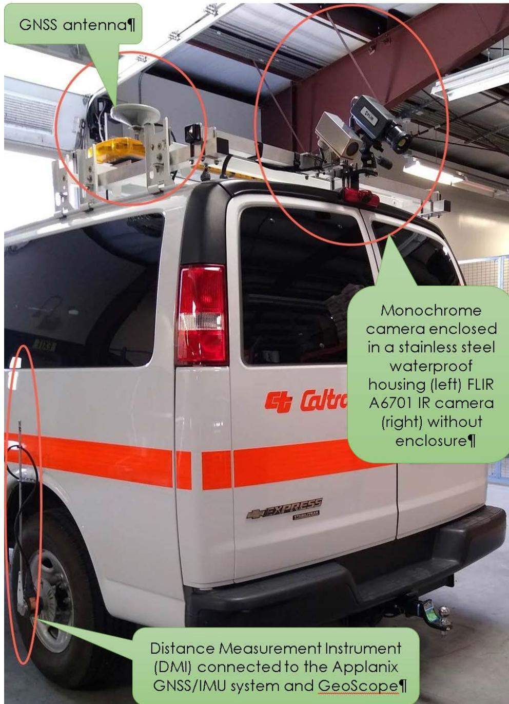
Figure 2.2: FLIR A7401 MWIR with 17 mm lens evaluation setup
