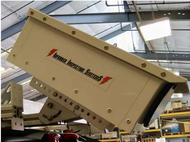
Figure 2.3: Mid-State Instruments FLIR IR camera enclosure (exterior view)
