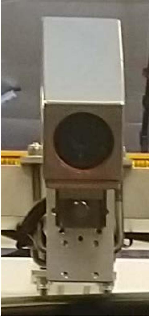
Figure 2.6: APG Vision model 30S-AD camera enclosure with the 30S-PT1 mount
