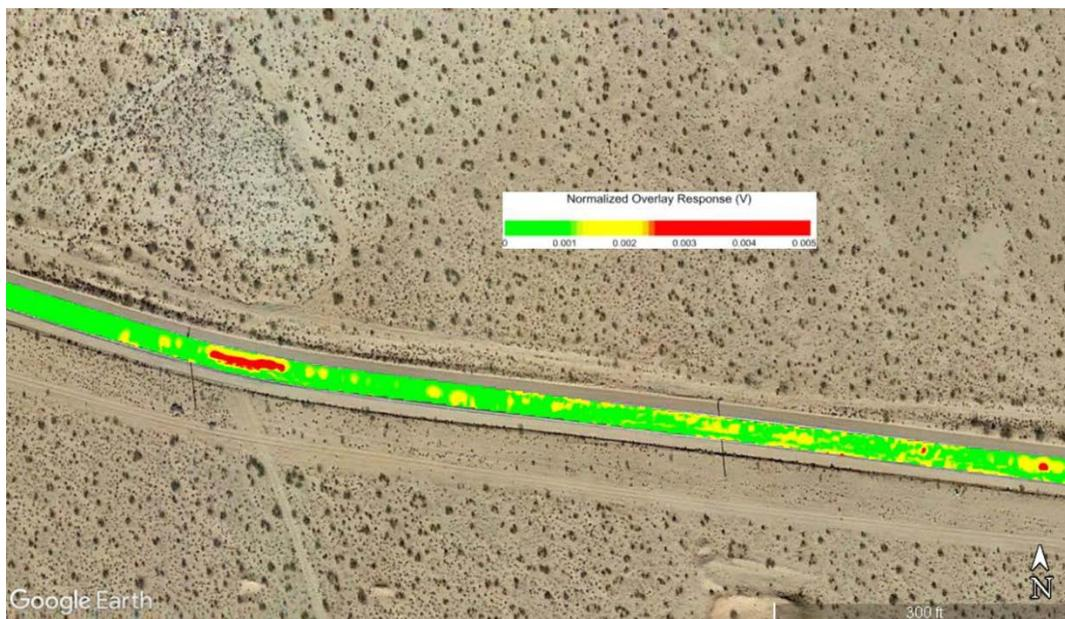
**Figure 1.1: A sample graphic of the pavement intralayer GPR response, which provides an indicator for overlay stripping or delamination**
