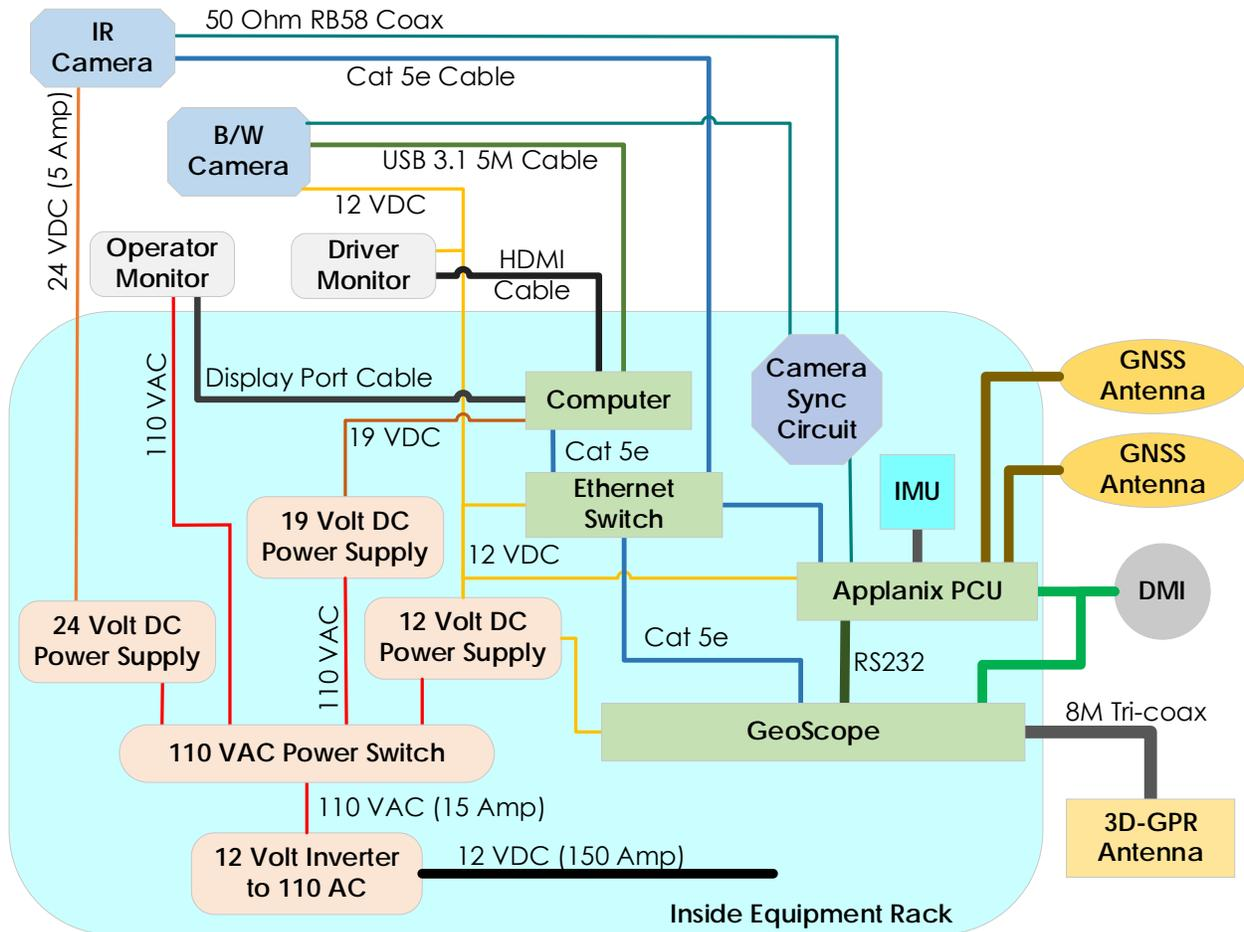
Figure 4.1: 3D-GPR system wiring diagram
