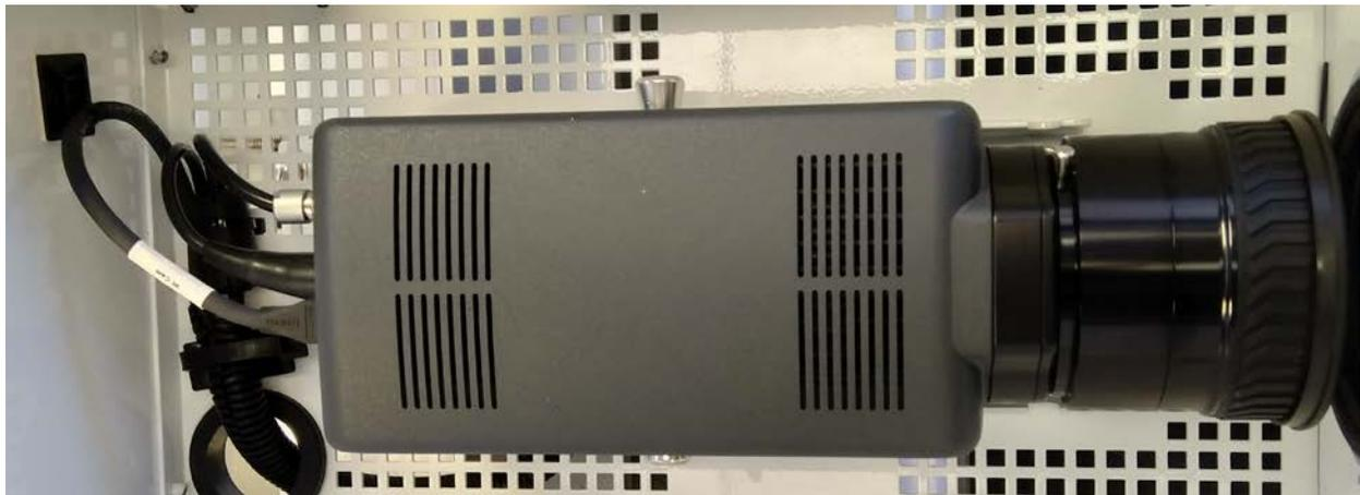
**Figure 2.1: FLIR A7401 MWIR with 17 mm lens (top view)**
