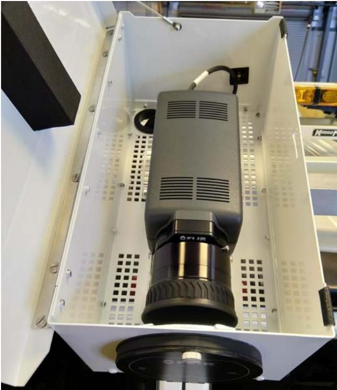
Figure 2.4: Mid-State Instruments FLIR IR camera enclosure (interior view)
