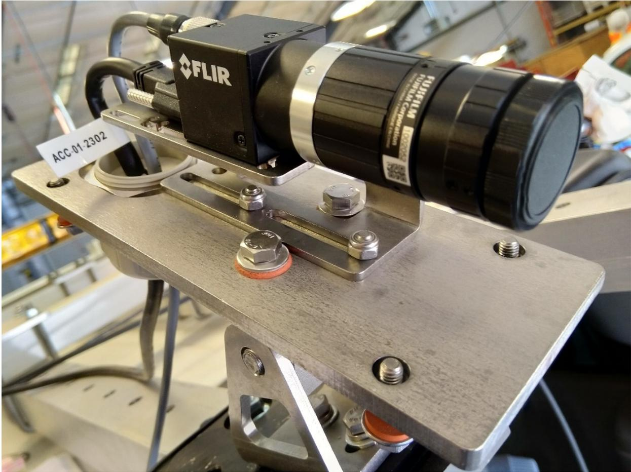
Figure 2.5: FLIR monochrome camera mounted inside the APG Vision model 30S-AD camera enclosure (the enclosure lid moved)
