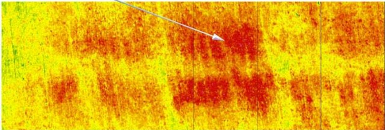
**Figure 1.2: A sample of a processed thermal image of a bridge deck where the color difference (red shade) can indicate delamination [1]**
