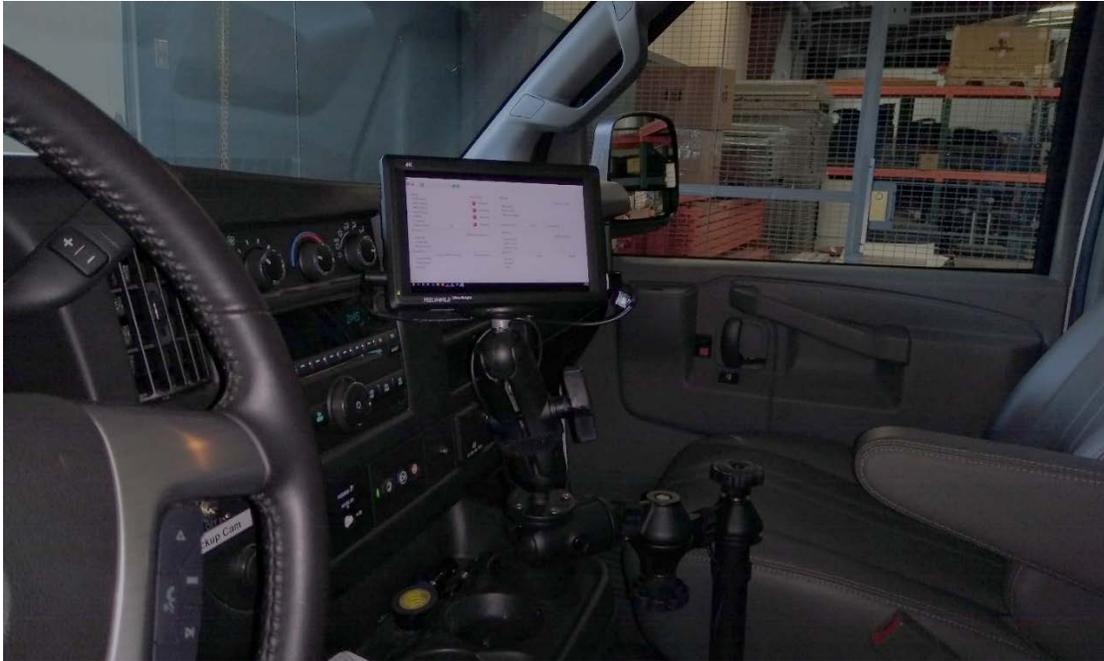
Figure 3.2: 7" 1080p driver guidance display
