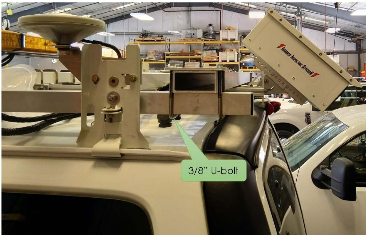
Figure 5.2: IR camera mount (side view)
