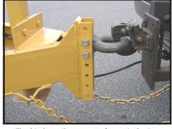
The hitch easily converts from pintle ring to ball, and provides generous height adjustments.
