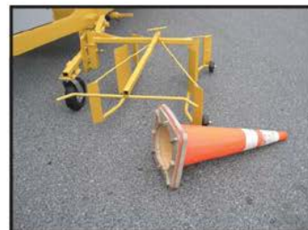
The machine will pick up cones that are still standing, or have been knocked over. The guide positions and feeds the cone where it is needed.
