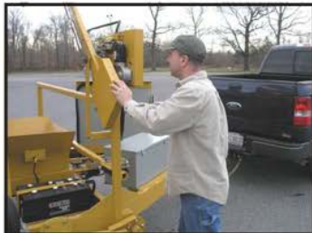
The machine will place and pick up cones from either side of the trailer. Moving from one side to another is simple and takes seconds.
