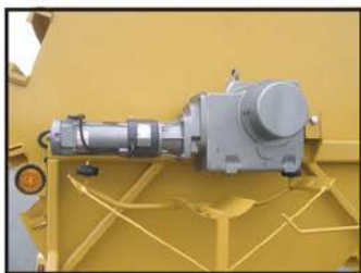
The entire cone storage drum rotates as needed to supply or retrieve cones. This rugged heavy duty gearbox handles the job with ease.
