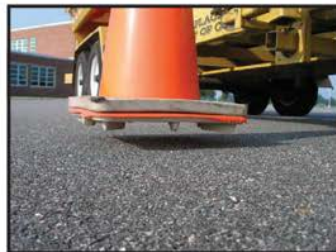
The cone hangs – waiting to be dropped on the road as you drive along. A simple button press drops the cone where you want it. The "hang height" is adjustable to accommodate road conditions and trailer hitch heights.
