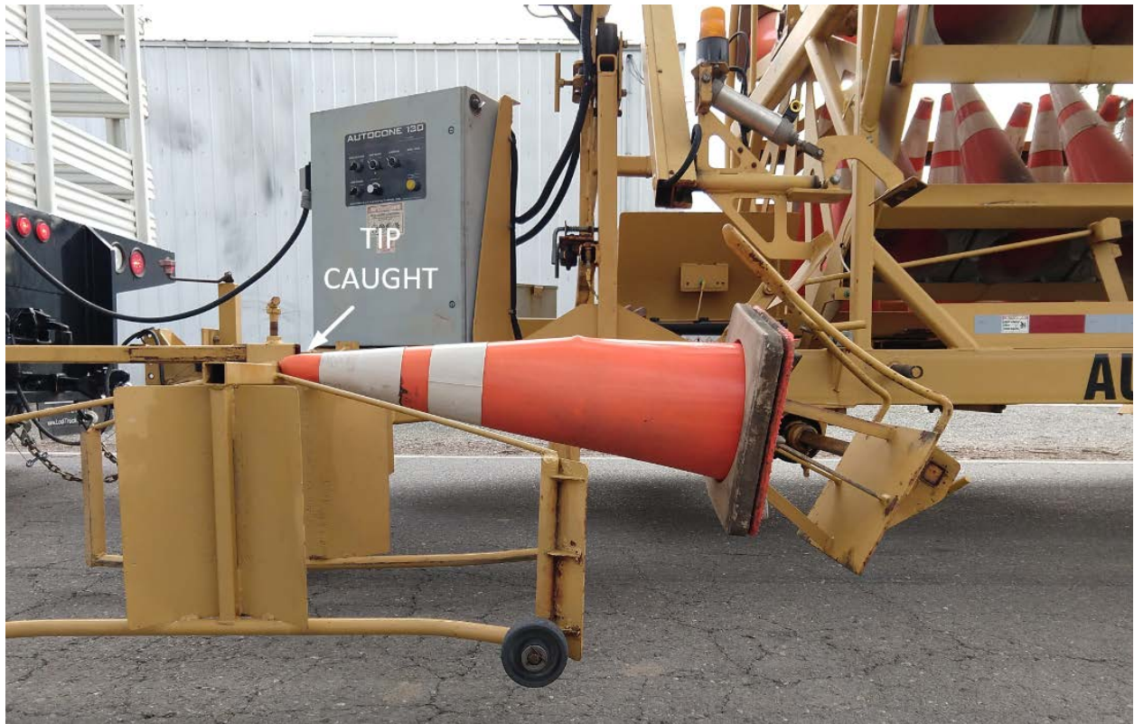
Figure 2.13: Retriever jam at low temperature
