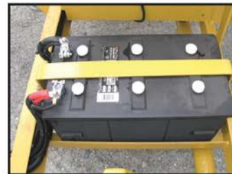
The machine operates on 24vdc power. The batteries shown allow the trailer to be totally self contained allowing any available truck in the fleet to do the job.
