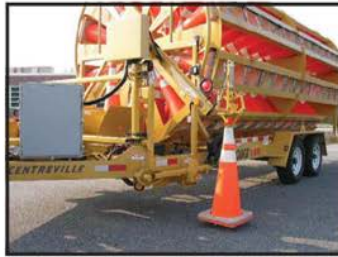
The machine holds 130 standard 36" cones with base weights attached.
