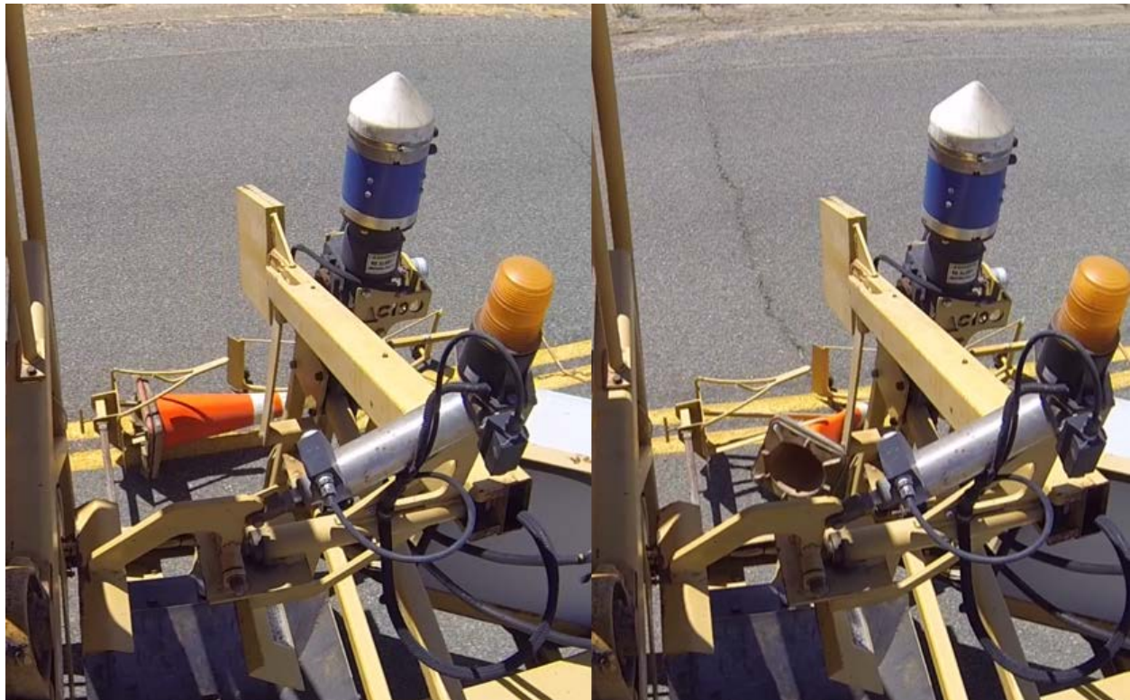
Figure 2.12: Normal retrieval (left) and jammed (right)
