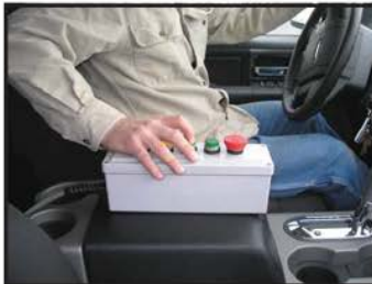
The driver controls the machine using simple controls, usually just one button push per cone.
