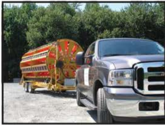
The machine tows using a 3/4 ton pickup truck. No modifications are required on the truck.
