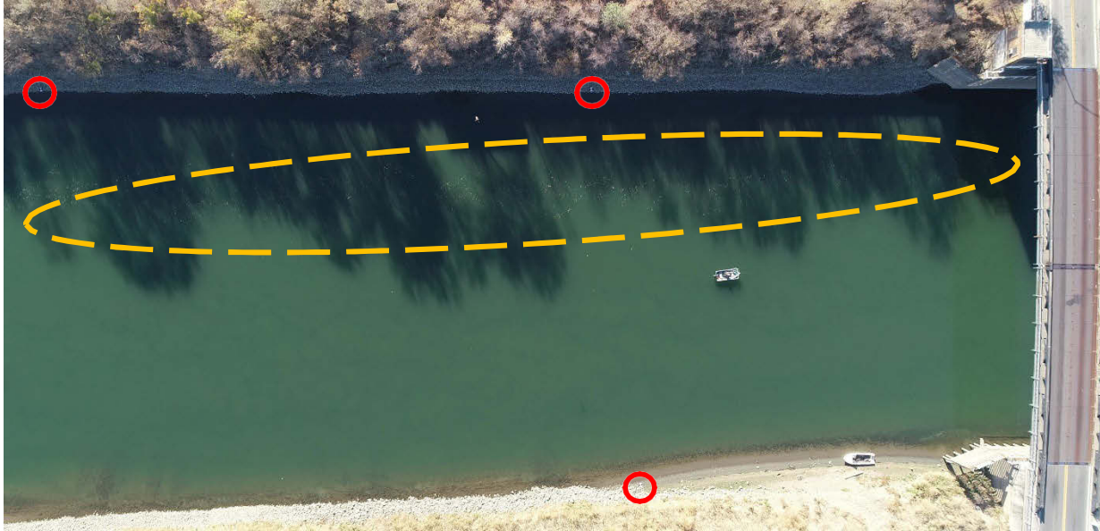
Figure 4.13: Example LSPIV 4K color video capture frame. Area with good, natural seeding is highlighted by a yellow dashed line, and red circles highlight the GCP targets.
