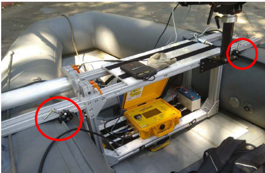
Figure 3.10: Component mounting platform secured in the Caltrans foldable boat with four clamps. Two of the clamps are visible and highlighted by red circles.
