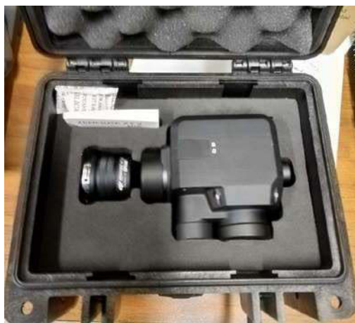
Figure 2.3: FLIR XT2 IR and color camera
