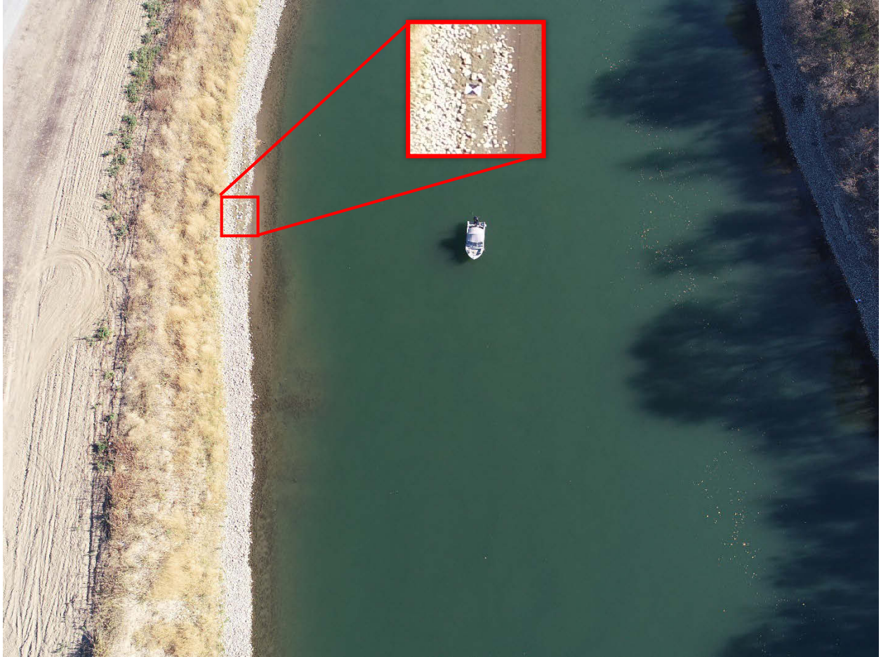
Figure 4.3: Example aerial image for topographic mapping. A GCP target (24" x 24") is highlighted with a red square.
