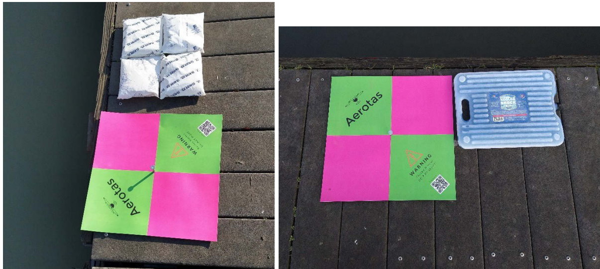
Figure 4.5: Aerotas 16" x 16" biodegradable GCP targets next to ice packs (10" x 13") used as thermal imaging GCP targets
