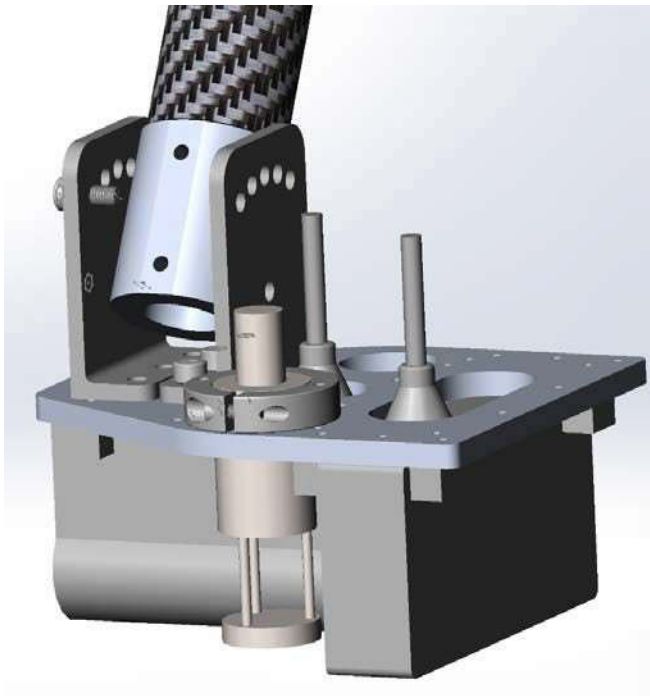
Figure 3.4: PicoMBES 120 sensor assembly with cover CAD model
