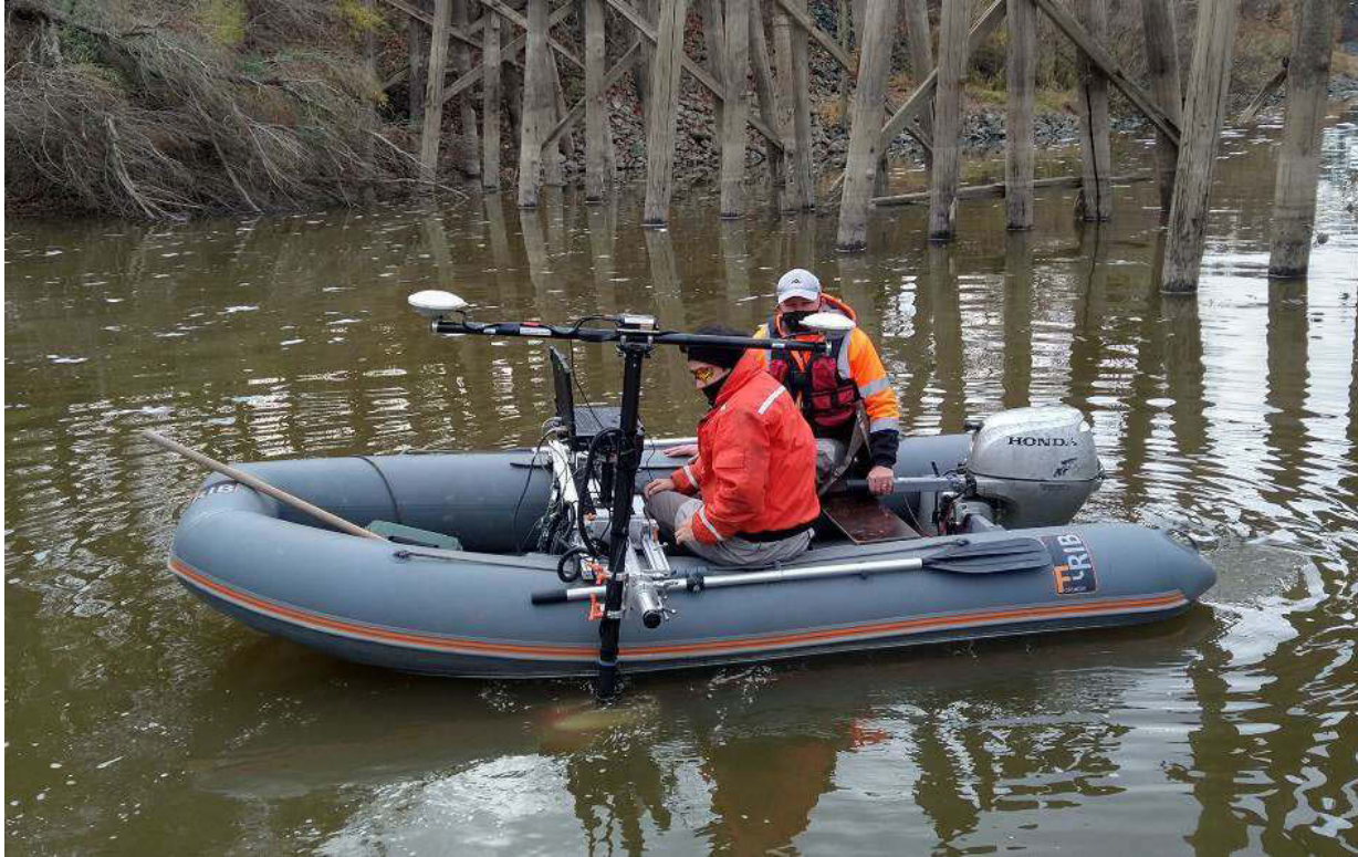
Figure 3.18: SM&I personnel testing the ADCP and echosounder integration with WinRiver II software. ADCP and CEE Echo sounder sensors are under water.
