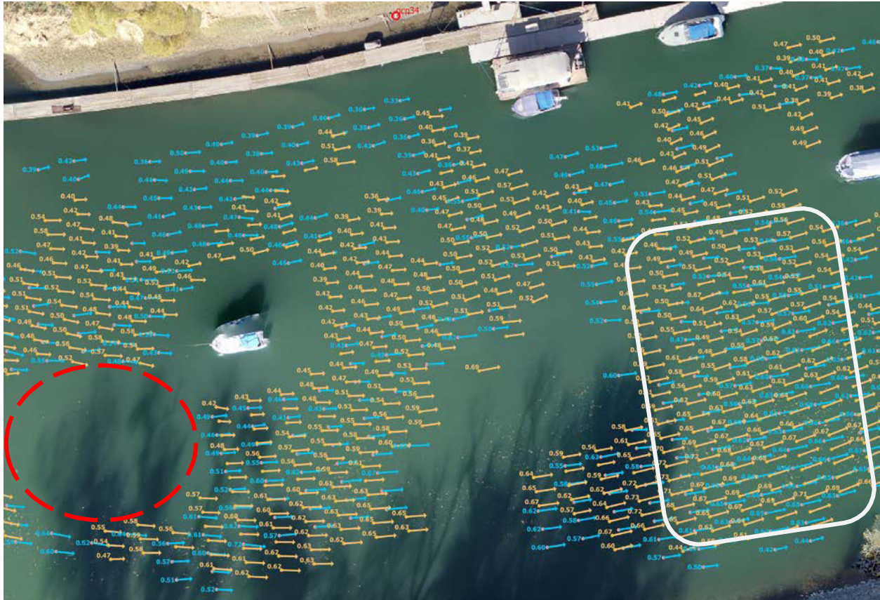
Figure 4.11: RIVeR LSPIV result overlaid on georeferenced orthophoto in QGIS. Area with good natural tracers is highlighted by a white rectangle, and area with poor/no natural tracers is highlighted by a red circle.
