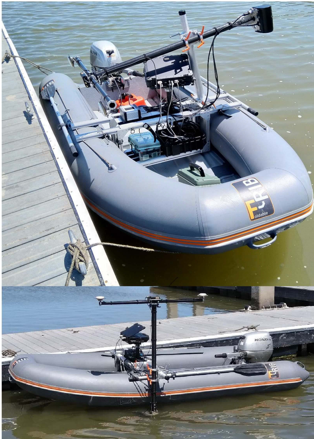
Figure 3.12: PicoMBES testing on Caltrans boat at Napa River (05/22/2020). The top photograph shows the sensor mask pivoted up so that the PicoMBES sensor is out of the water (transit configuration).
