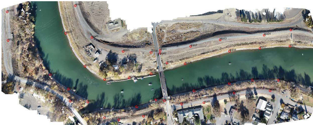
Figure 4.2: SR113 pilot study site Ground Control Points (GCP) overlaid on top of orthophoto created by WebODM
