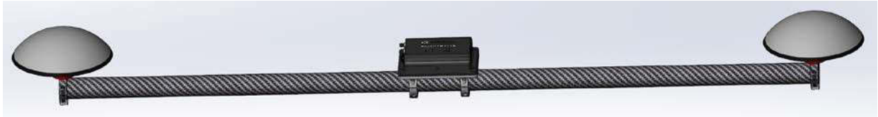
Figure 3.1: Advanced Navigation Spatial Dual GNSS/IMU positioning system SolidWorks sub-assembly CAD model
