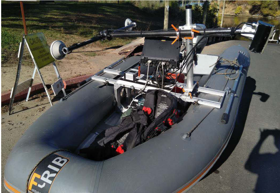
Figure 3.9: SM&I foldable boat with PicoMBES 120 with 15-degree tilt at Discovery Park boat launch (10/15/2020). The sensor mask is rotated up before transit to into water.
