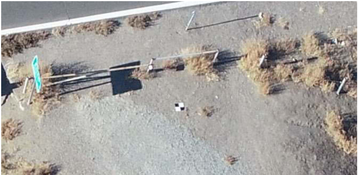
Figure 4.4: Cropped aerial image with a 12" x 12" GCP target
