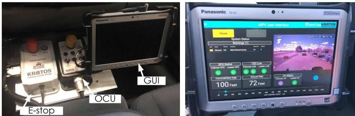
**Figure 3.4: ATMA LV user interface controls**
