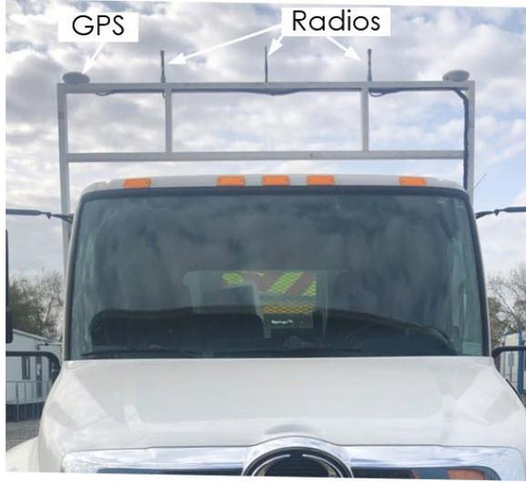
**Figure 3.6: FV antenna rack**
