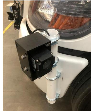
**Figure H.3: Upgraded side LiDAR sensor**
