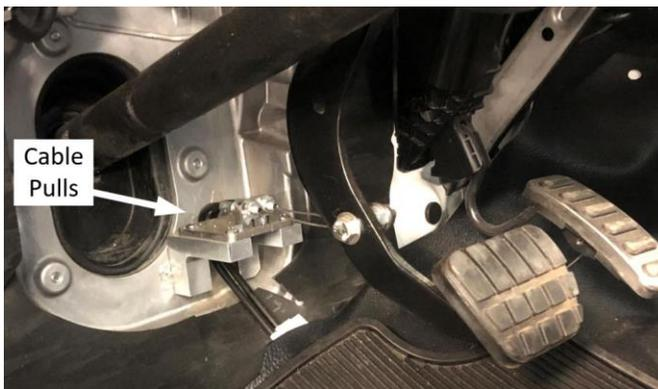
**Figure 2.3: Brake cable pulls**
