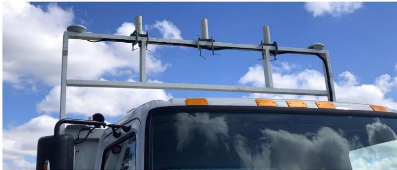
**Figure 3.10: Temporary radio antenna guards**
