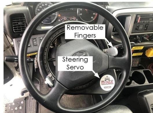
**Figure 2.4: Steering motor**
