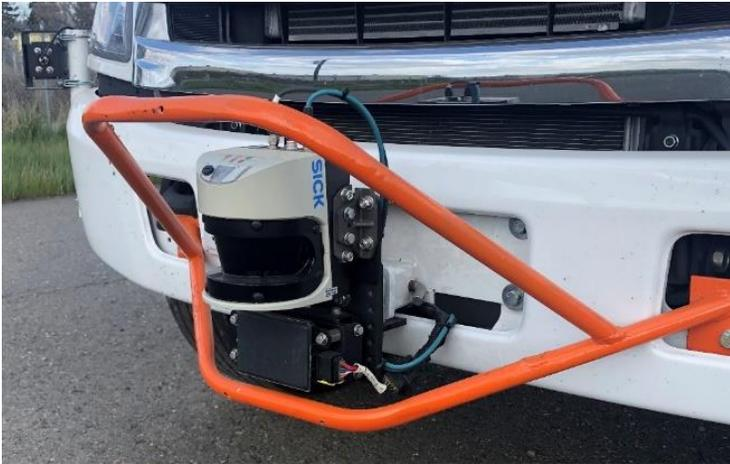
**Figure H.2: Upgraded LiDAR sensor**
