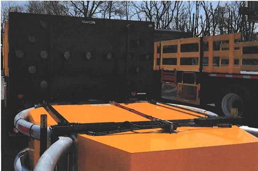
Figure 15: Stowing the Arrow Board
