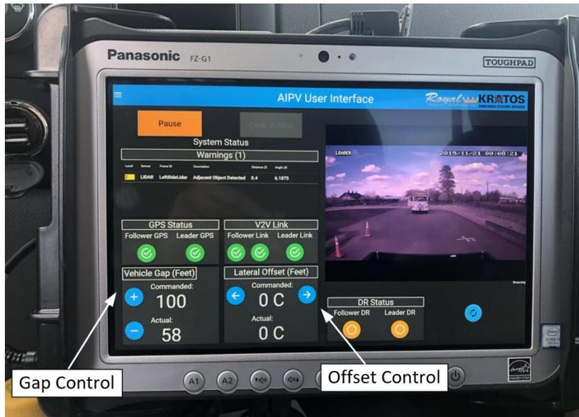
**Figure 2.6: LV GUI offset and gap controls**
