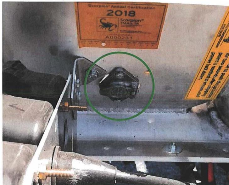
Figure 12: Auxiliary Controller Plug
