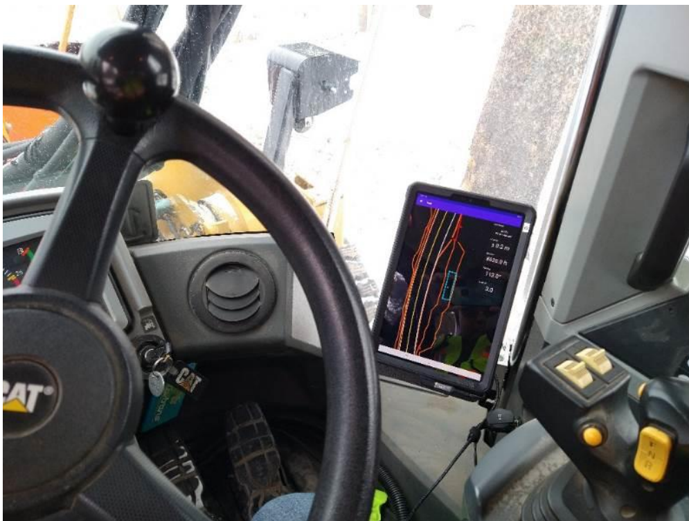
Figure 6: Updated MPRO system installed in front-end loader. This clearly illustrates the greatly improved sunlight readable capability of the final system.
