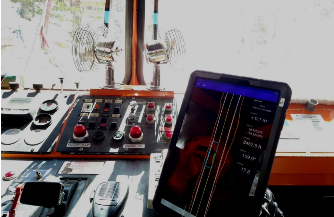
Figure 5: Updated MPRO system installed in rotary snow blower. This clearly illustrates the greatly improved sunlight readable capability of the final system.
