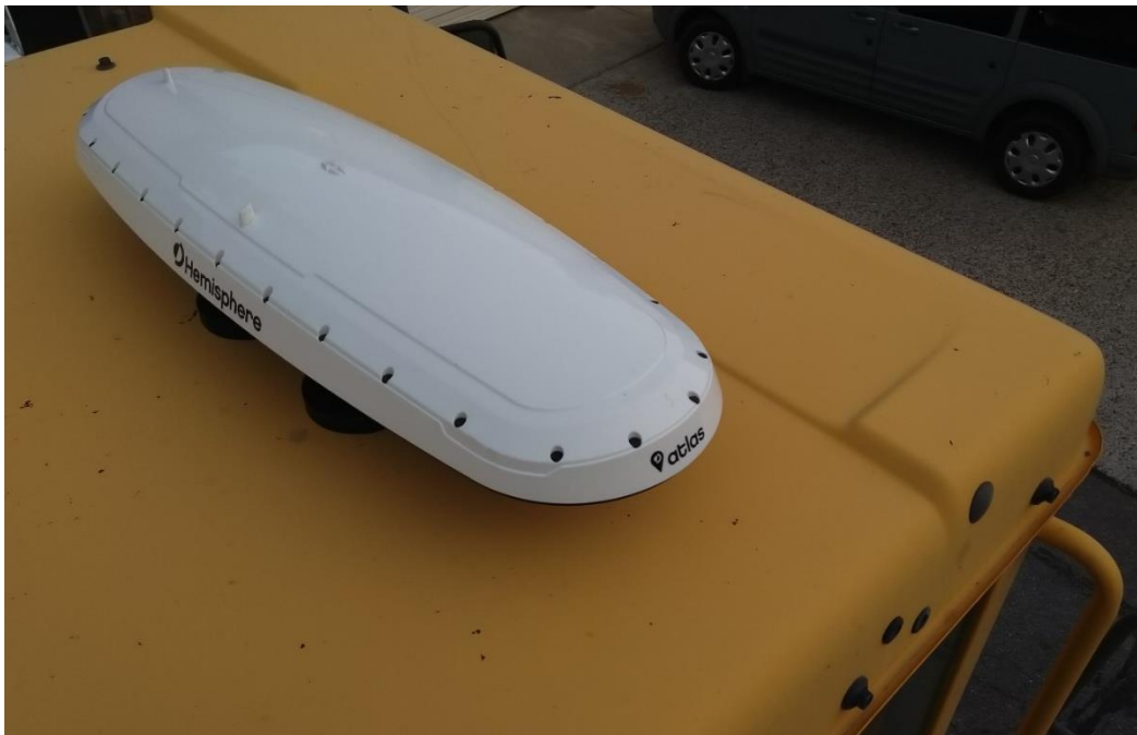
Figure 2: MPRO Hemisphere V500 Vector GNSS sensor mounted on top of a loader using magnetic mount
