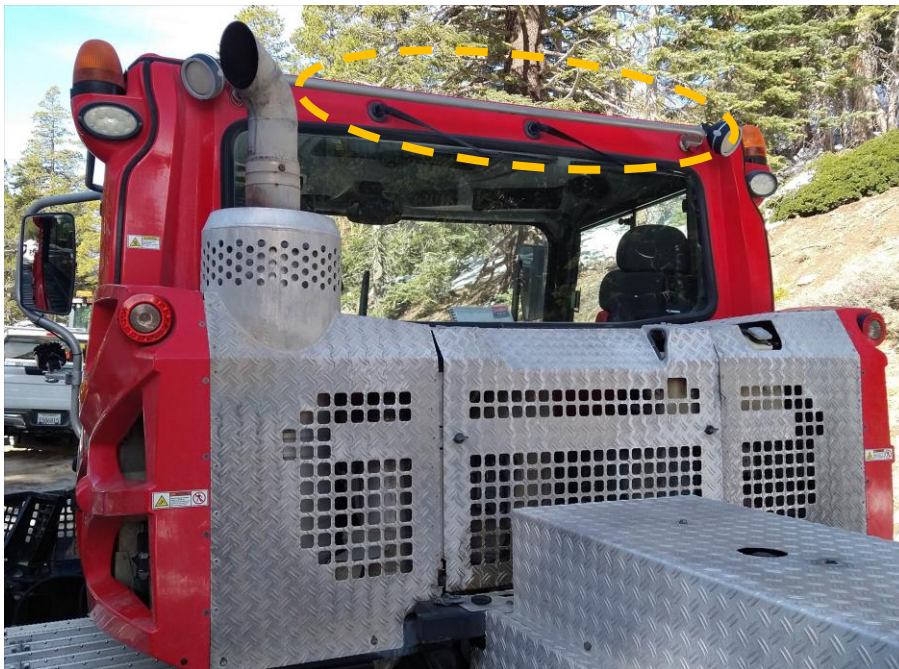
Figure 11: The PistenBully 400 1" handlebar (highlighted in yellow) near the top of the cab is suitable for the GNSS mount
