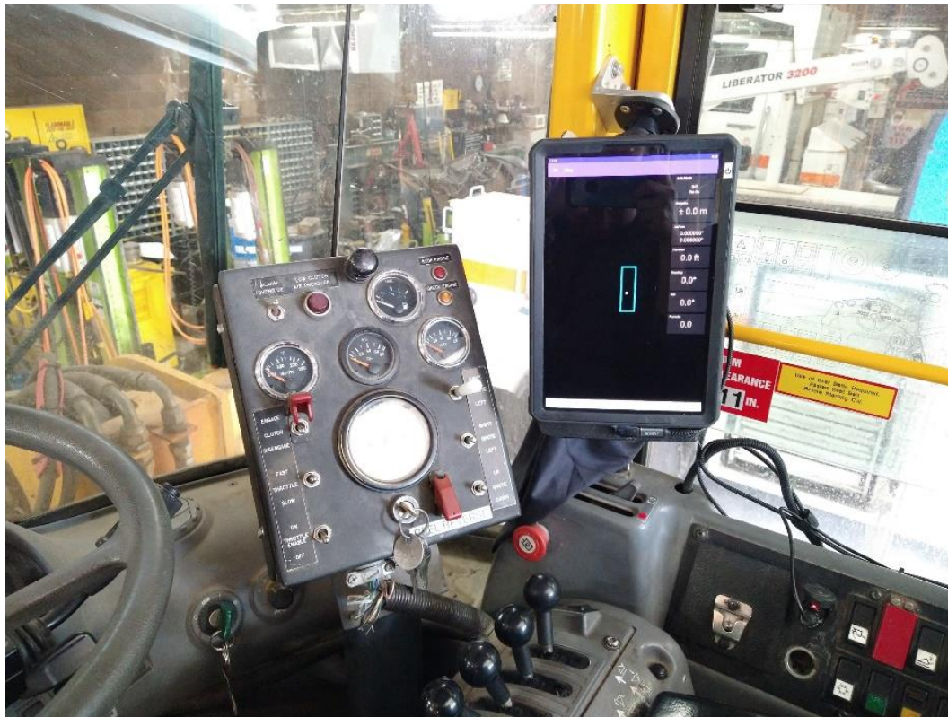
Figure 7: MPRO tablet installation on another front-end loader. The image was taken inside the shop building, hence the GNSS position is not available.
