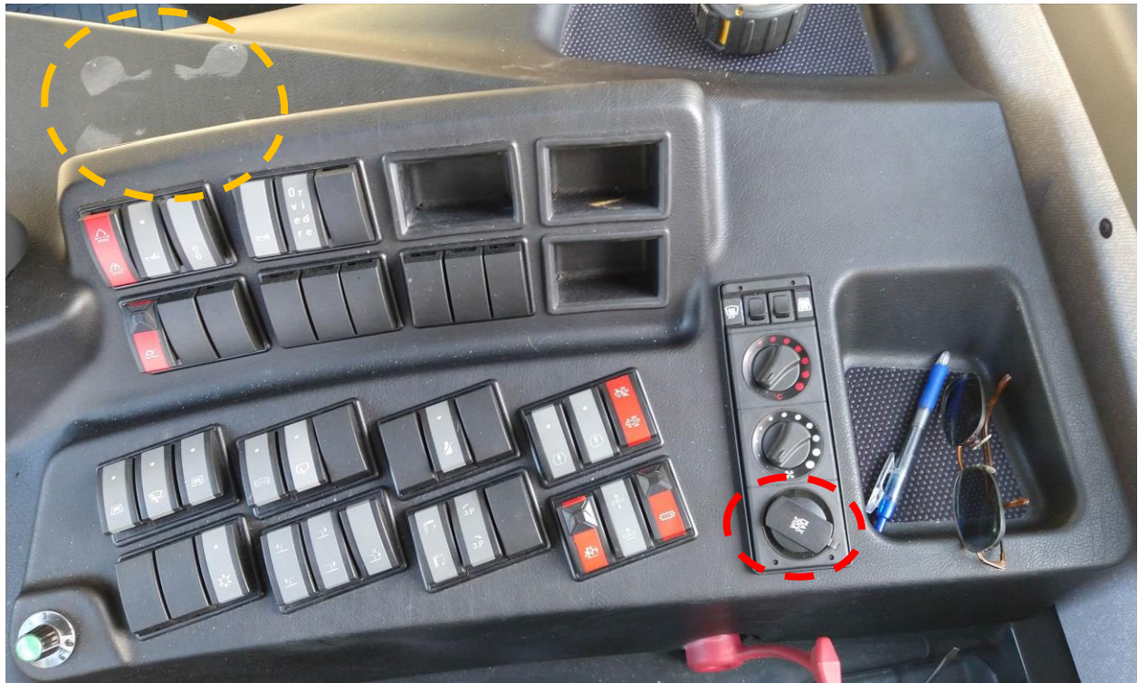
Figure 12: PistonBully 400 dashboard (right side of the driver seat). Table mount location is highlighted in yellow, and 12-VDC power outlet location is highlighted in red.
