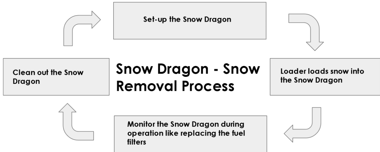
Figure 2.2: Snow removal process using the Snow Dragon
