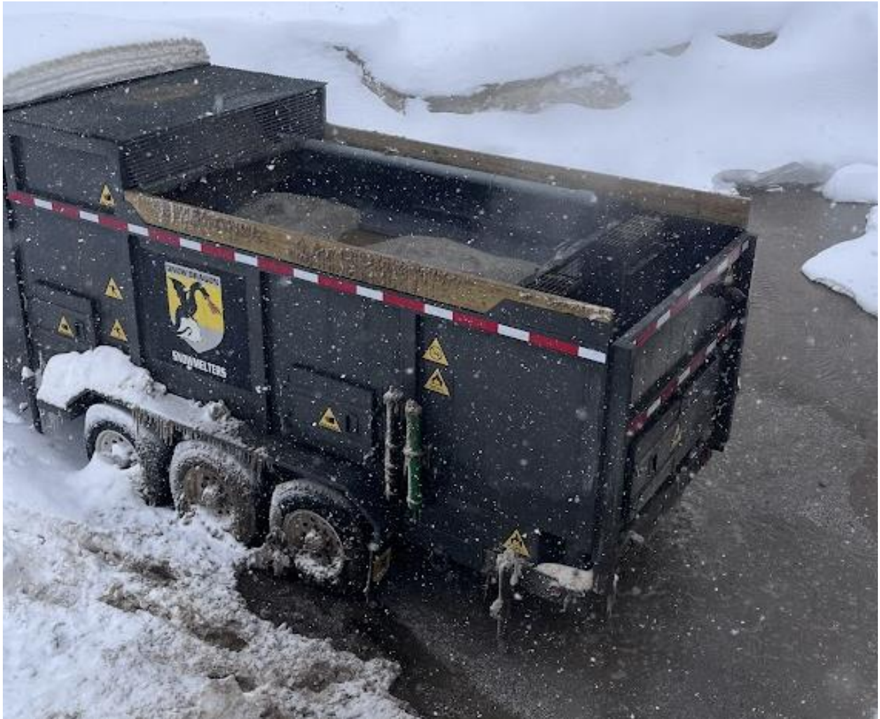
Figure 5.2: The top of the Snow Dragon and its condition after melting snow with more sand for 100 minutes straight
