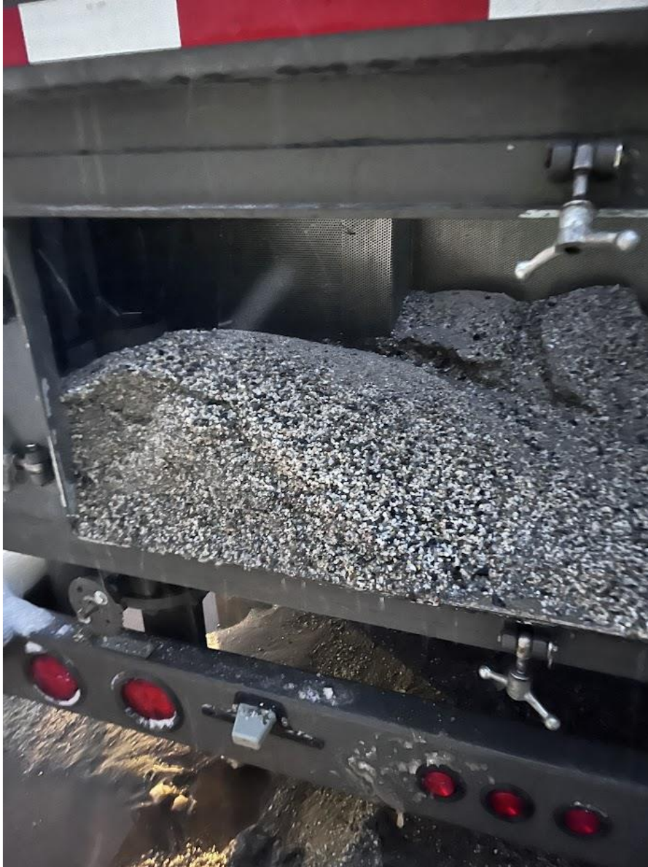
Figure 5.6: The bottom of the Snow Dragon and its condition after melting snow with less sand for 205 minutes
