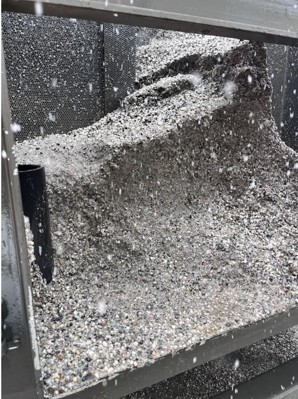
Figure 5.3: The bottom of the Snow Dragon tank and its condition after melting snow with more sand for 100 minutes straight
