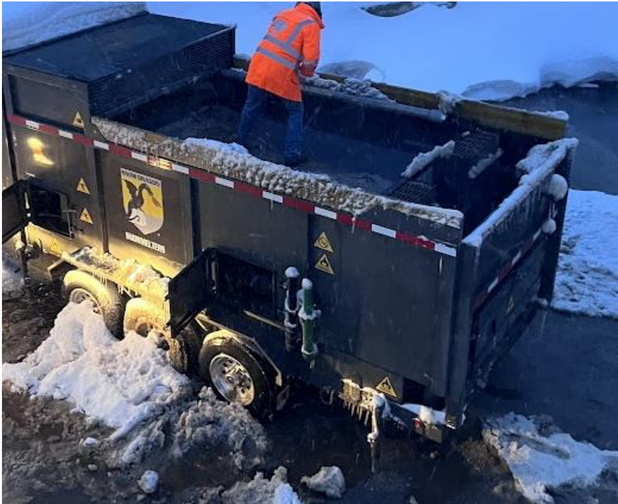
Figure 5.5: The top of the Snow Dragon and its condition after melting snow with less sand for 205 minutes
