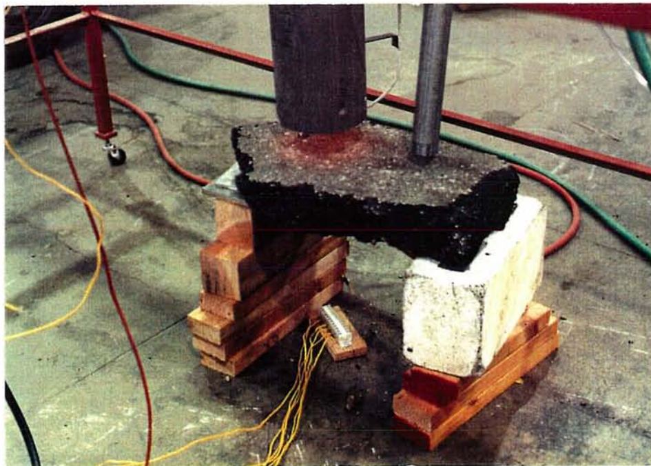
Figure 6.5 - Close up of sample being heated with Sur-Lite burner. Note: the thermocouples mounted in the sample were not used in this study.
