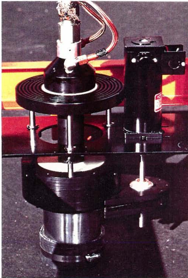
Figure 6.13 - Sealant Applicator Mounted in Longitudinal Test Cart.
