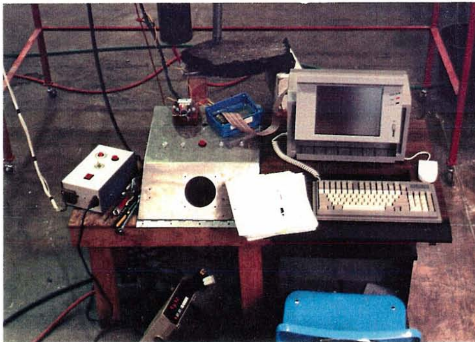
Figure 6.7 - Data acquisition station. The control box on the left provides power to the cart motor. To its right is the scrap panel that houses the spark ignitor push button and solenoid valve toggle switches for the burner. On top of it is the transformer providing 12 VAC power to the pyrometer and the connector board for the inputs to the DAS-16 card. On the floor a thermocouple is connected through a DVM to measure ambient temperature.
