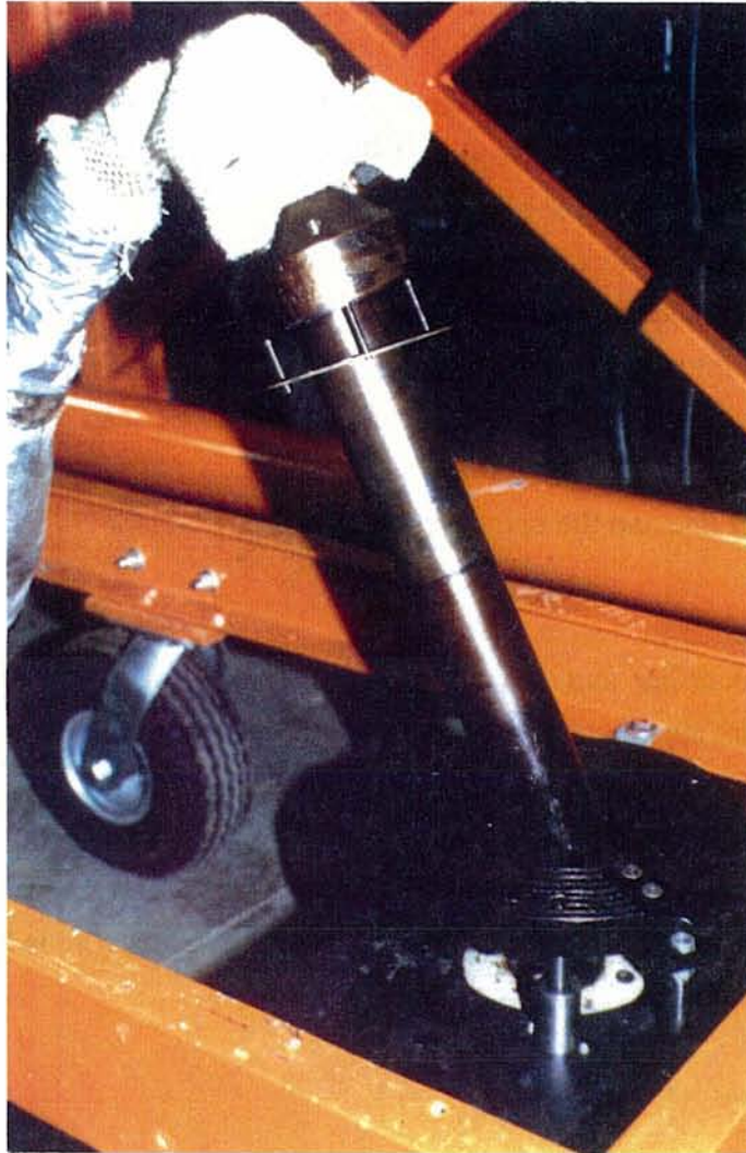
Figure 3.2.2 - Sealant Applicator Core Installation and Removal.
