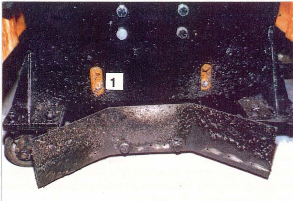
Figure 5.2.2 - External Router Sliding Block Retaining Bolts.
