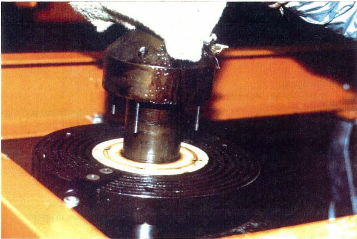
Figure 3.2.3 - Sealant Applicator Core Cap Installation and Removal.
